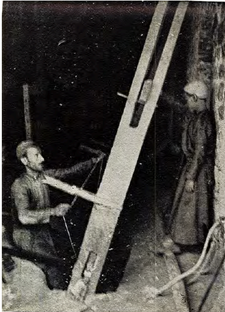
Figure 4.13 Image of a man weaving on a two-beam vertical loom in Syria, c. 1940. The bottom of the loom is in the pit as the man sits on the edge and the loom rests against the wall. Reproduced from Crowfoot 1941, pl. XII.I
