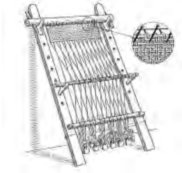
Figure 9 Depiction of a warp-weighted loom. Reproduced from Ciszuk and Hammarlund 2008, 122.
