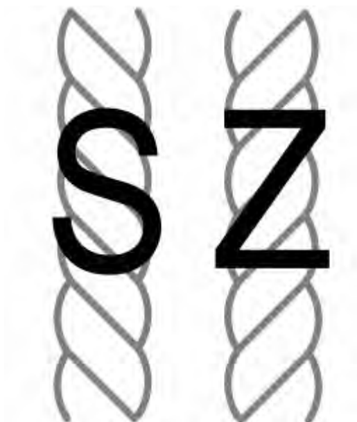
Figure 2.13 Diagram showing s-spun and z-spun threads. Reproduced from Wikimedia Commons
