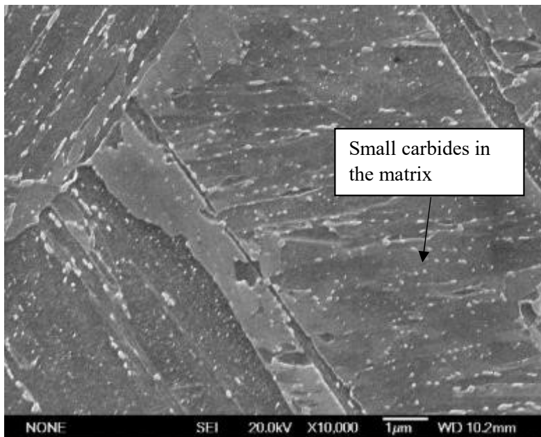
Figure 89 SEM micrograph showing carbides in the BaseMoV steel after 16 hours tempering at 600 °C (higher magnification) ( 321.3 \pm 8.0 HV)
