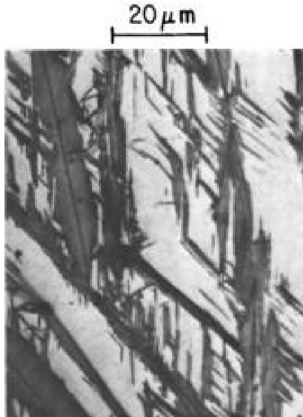
Figure 10 Structure of plate martensite in a 1.2 wt. % C steel (Speich & Leslie, 1972)
