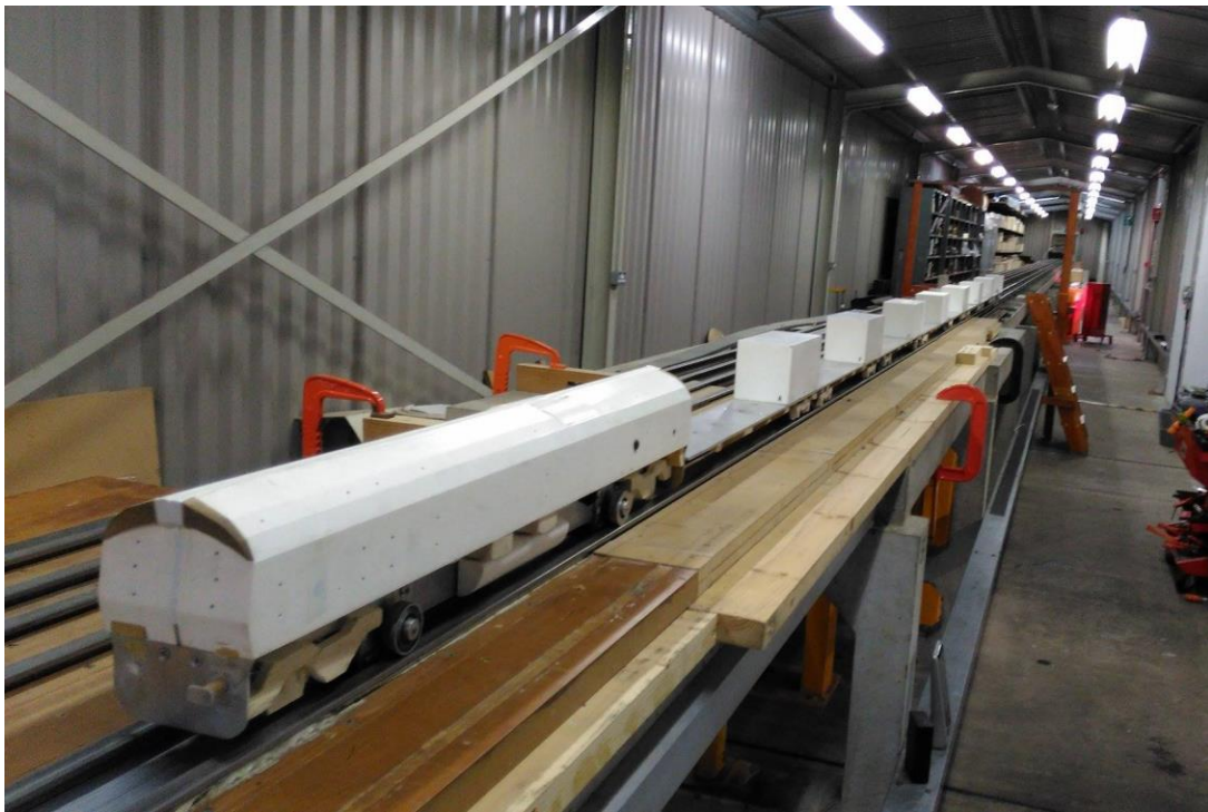
Figure 3.4: Partially loaded train (33%) with 8 wagons (case 3)
