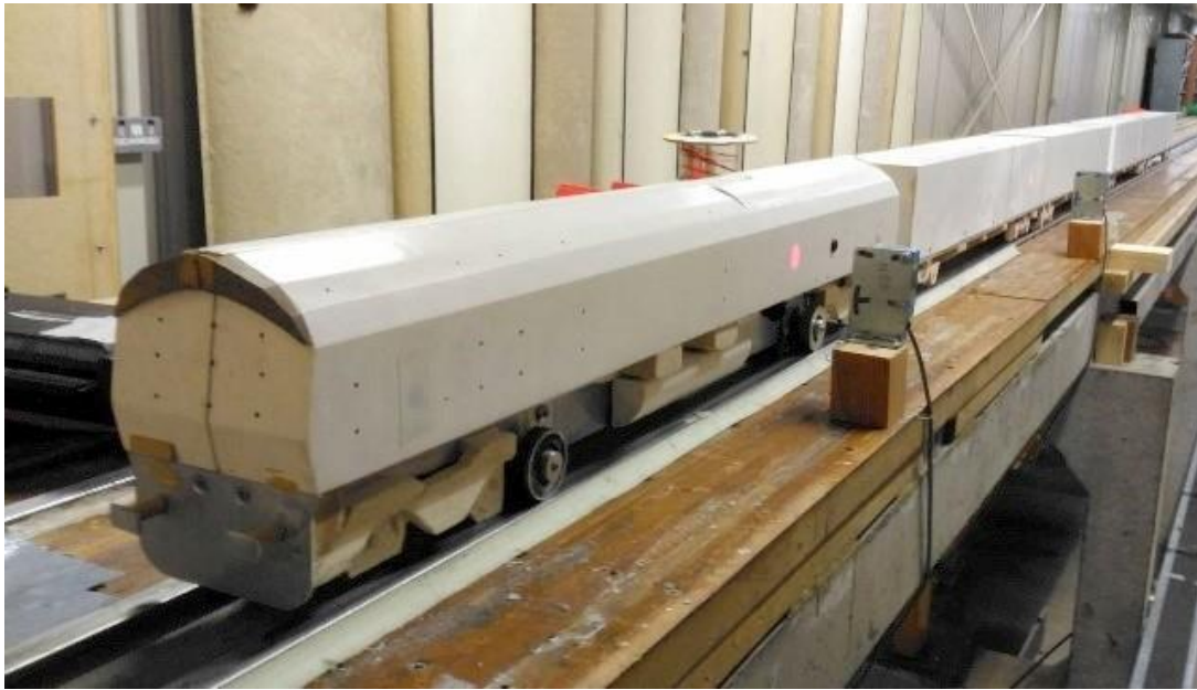
Figure 3.3: Model-scale locomotive connected to 4 container wagons (case 1). The locomotive surface is drilled to accommodate the pressure taps.
