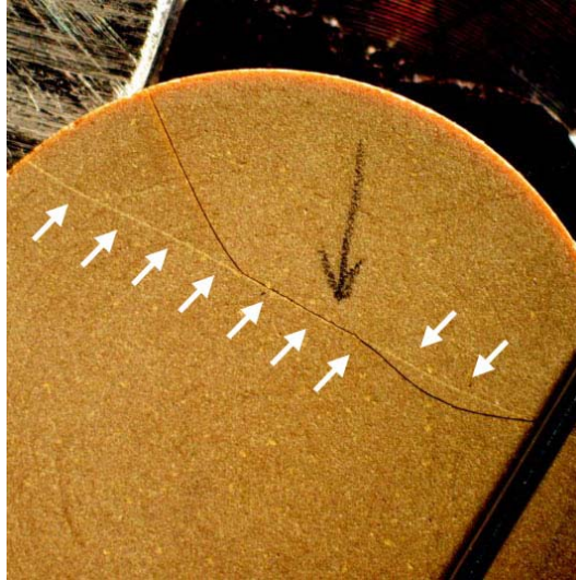
Figure 8-14 Example of a surface scratch acting as a fracture origin. The primary fracture plane clearly follows a portion of the scratch.
