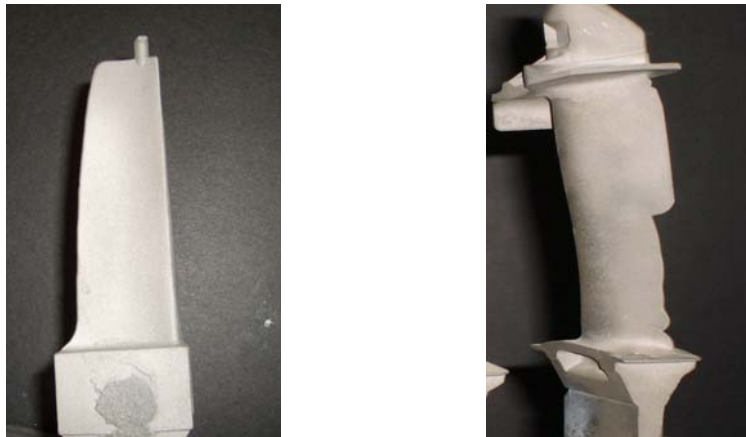
Figure 1.2 Misrun defects in thin section turbine blade castings
