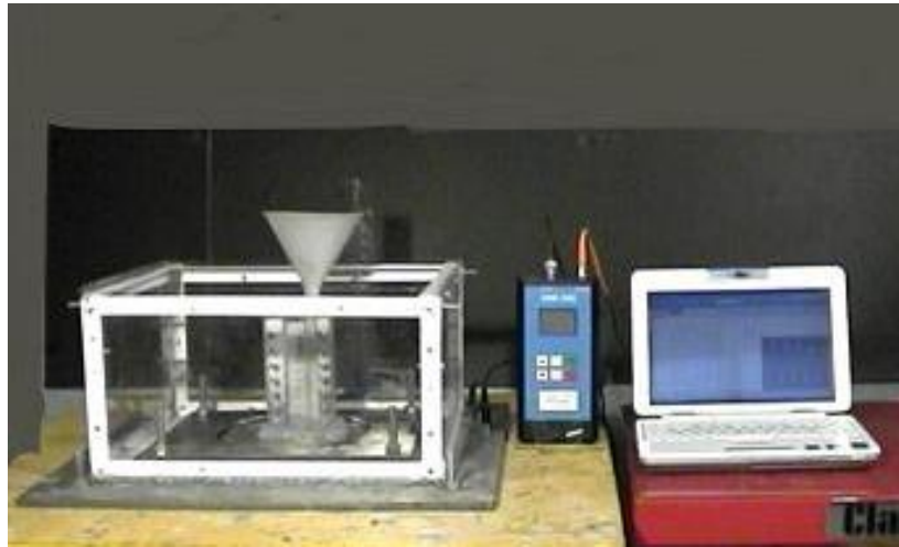
Figure 3.20 mercury experimental to investigate the liquid metal advance and velocity of the metal under vibration condition
