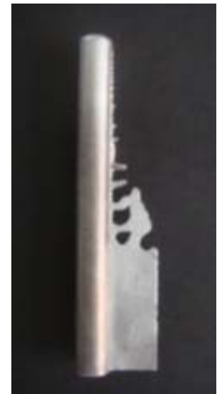
(c) a jetting length at 1.2g acceleration of vibration
