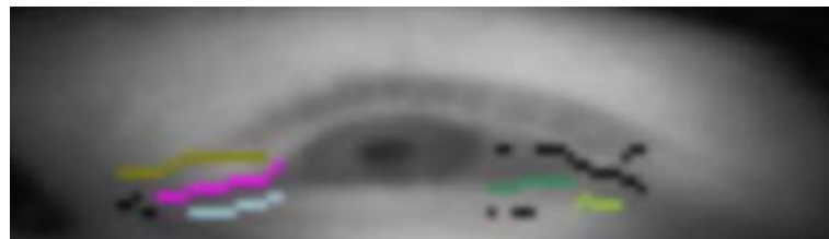
GROUPINGS GENERATED BY APPLYING A DISTANCE CRITERION TO LOCAL MAXIMA OF THE Y-DERIVATIVE IMAGE AFTER NON-MAXIMA HAVE BEEN SUPPRESSED (SCALED UP X4)
