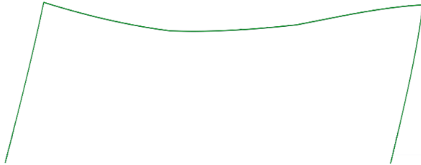
Fig. 6.11: Combined plastic mechanism of a pin-ended frame
