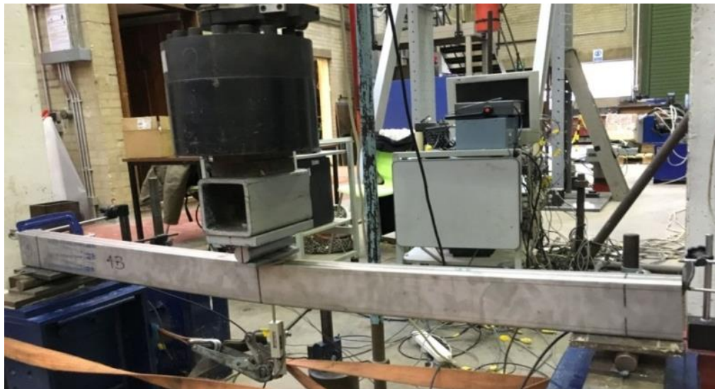
Fig. 3.5: Overall setup for 3-point bending tests
