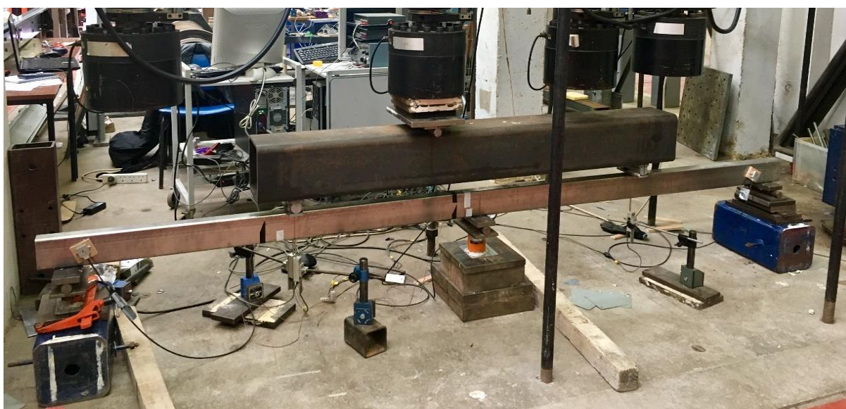
Fig. 3.9: Overall setup for continuous beams
