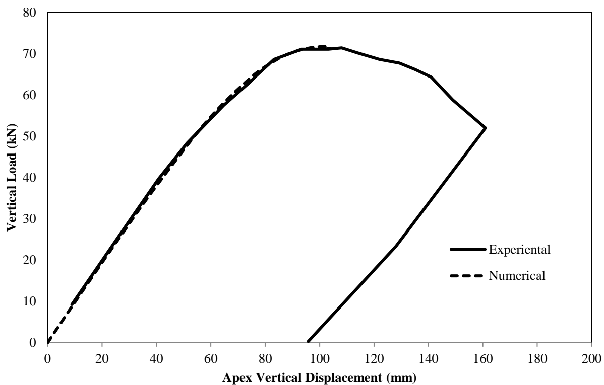
Fig. 5.21: Vertical load – vertical displacement apex for Frame 2
