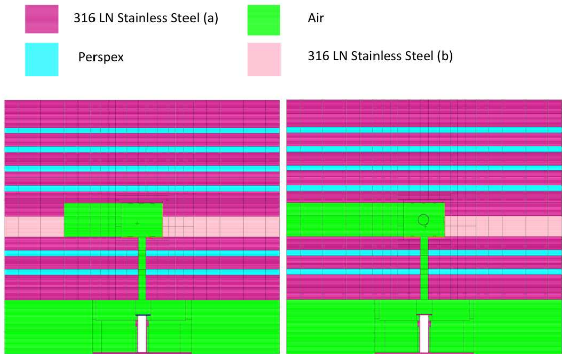
Figure 5.12: MCNP models for the irradiation (left) and decay (right) simulations and the material distribution shown by the colours
