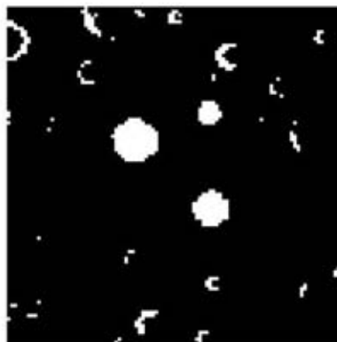
Figure 8.18 Filling the voids within the in-plane bubbles.
