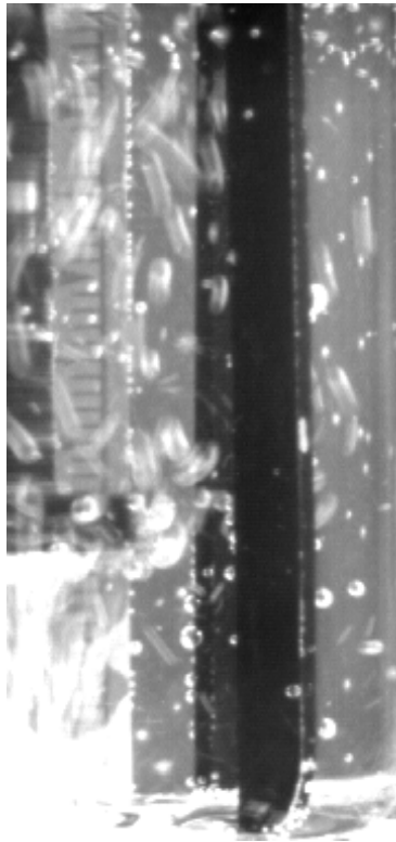
Figure 8.25 Captured from high speed camera (100fps) footage showing spatial distribution of bubbles at Q_G = 0.5 vvm: bubble streaking can be seen beneath the impeller and around the shaft where gas velocities are highest consistent with PIV measurements determined from new image processing algorithm.
