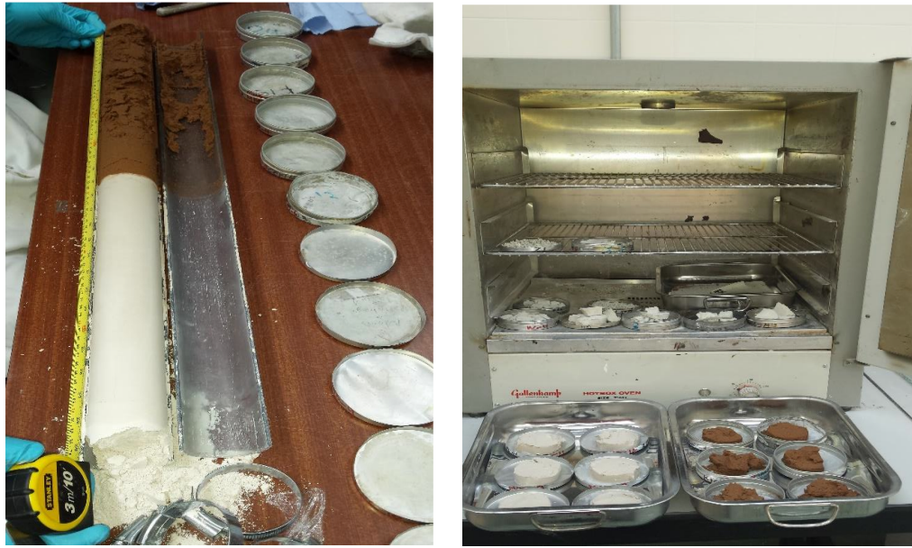
Figure 3.6 Soil sample preparation for the measurement of gravimetric moisture content.
