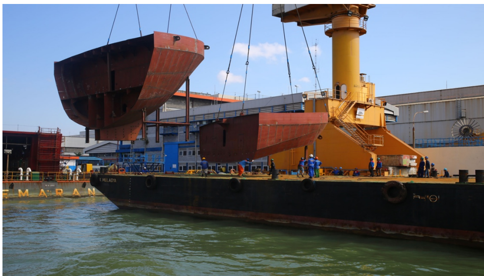
Figure 4.3. Cranes lift sections of the vessel onto the assembly dock
