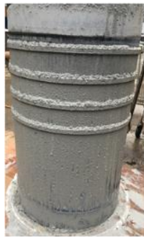
c) Dismantled sleeve after grouting during trials
