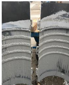
c) Dismantled sleeve after grouting during trials
