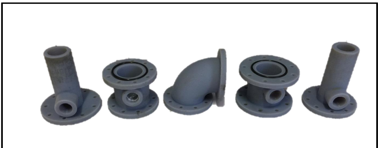
Figure 5-9 Pictures of the manufactured test rig pipe fitting.
