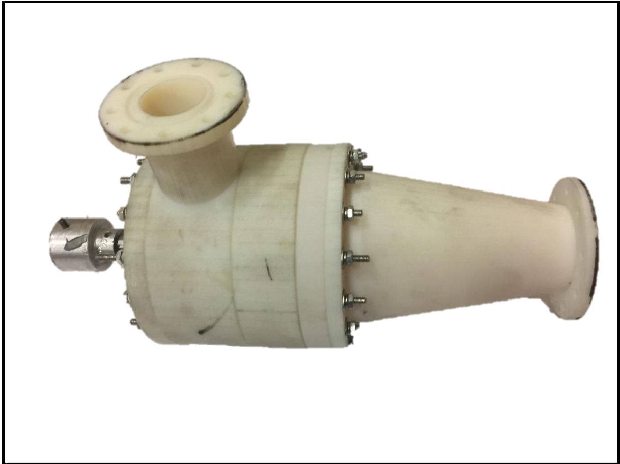
Figure 5-8 Pictures of the manufactured assembled small-scale turbine.
