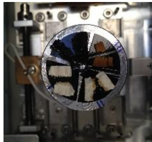
Figure 3.10 Picture of sample prepared for SEM observation.
