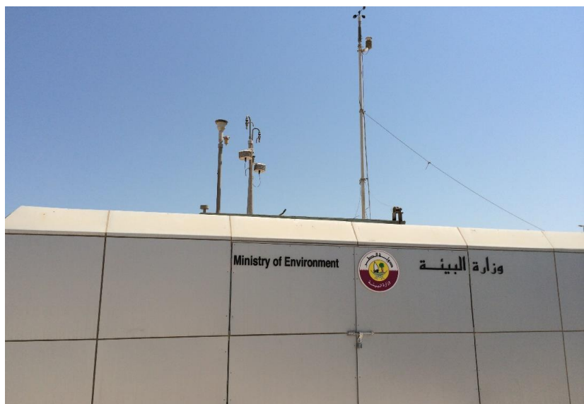
Figure 2.6 Samplers' goose-neck inlets at the height of 4 m above ground level
