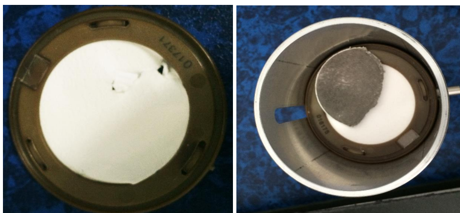
Figure 2.4 Damages to quartz filters during disc rotation
