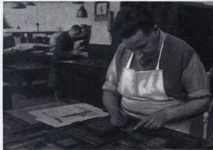
3 The Type Matter is Made Up After the first proof has been checked through by expert readers and the metal type corrected, it is put into formes and built into the exact position it will occupy on the page.
