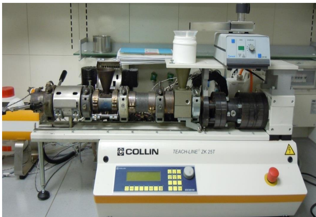
Figure 2-8 Laboratory extruder used to produce ABS solid reference material
