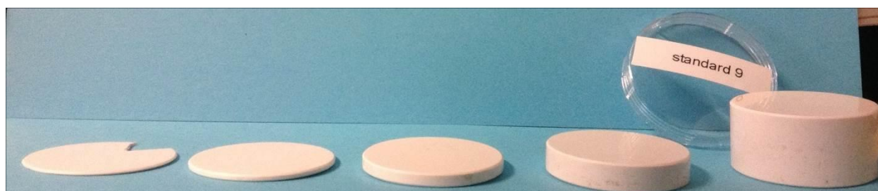
Figure 2-9 Discs of BDE209-loaded ABS. 5 pucks of different thicknesses were produced for each of the 9 concentration levels
