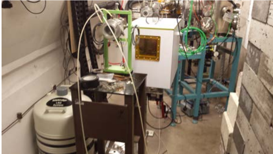
Figure 3.14: The current state of the University of Birmingham irradiation facility after the installation. The dewar containing the liquid nitrogen used in the process can be seen to the left.
