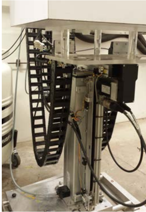
Figure 3.4: Photograph of the electronic mount that moves the cold box.
