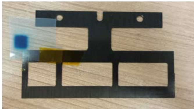
Figure 3.2: Long 'strip' frames designed to hold long-sensors.
