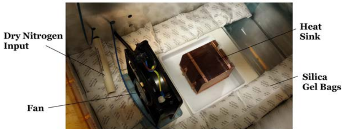
Figure 3.13: Interior photo of the new cold box. Electric fan seen to the left. Heat sink to the right, placed directly underneath liquid nitrogen input. Edges of the box have been packed with silica gel bags to further reduce humidity inside the box.
