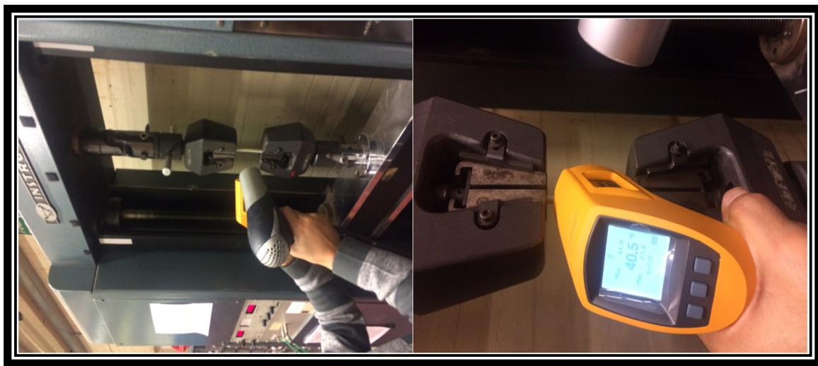
Figure 6.17: Tensile test carried out for three examined materials; at 40 °C.
