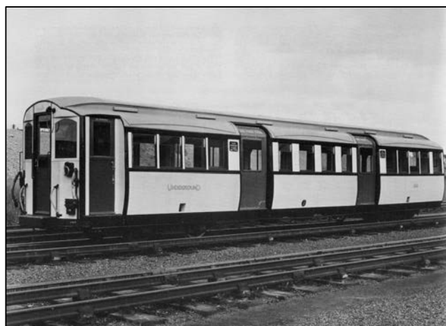
Figure 43: A CLR control trailer car after its conversion to air operated doors. The end platforms were fully enclosed and two single doorways were cut into each body side. The conversion of these wooden-bodied cars was much easier than for the steel-bodied LER cars. The doors were controlled through a compressed air control pipe operated from the guard's position by a special valve, rather like a brake valve. Collection: Author.
