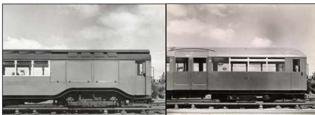
Figure 26: Side views of old and new tube car designs. On the left, the switch compartment end of a 1931 Stock motor car with the raised floor over the motor bogie. On the right, a 1938 motor car showing how the switch compartment area has been removed in favour of passenger accommodation by introducing small motors and traction control system. Photos: LT Museum.
