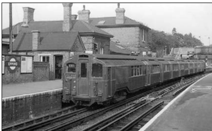
Figure 25: A 4-car train of Standard Tube Stock at Epping about 1957. The four cars are each from different orders ranging from 1923 to 1926. It was during this period that the Underground tried alternative suppliers
