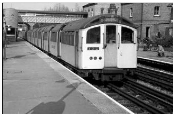
Figure 71: A 7-car train of 1959 Tube Stock at Woodside Park in the late 1970s. A large fleet of these and very similar 1962 Tube Stocks were built for the Central and Piccadilly lines. This was the first production stock built with rubber suspension. The '59 Stock began moving to the Northern to replace 1938 Tube Stock when the Piccadilly line began getting new 1973 Tube Stock.
