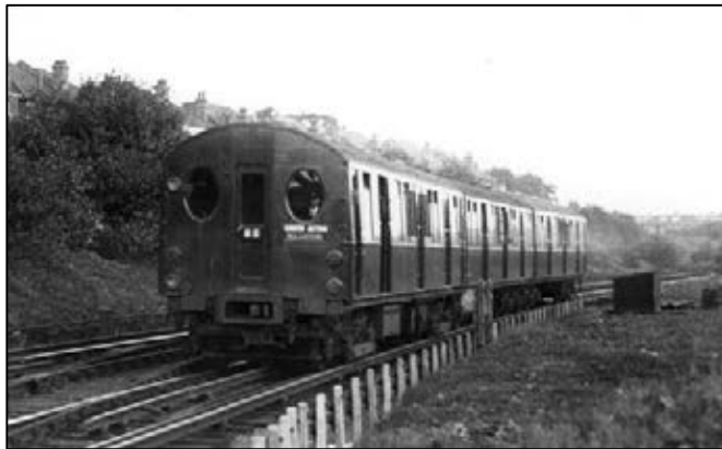
Figure 24: This is an early photo of the District's 1920 Stock, which later became known as the F Stock, under London Transport's management. A hundred cars of this stock were bought as part of an intended upgrade for the District. Motor cars were originally 'double-equipped', i.e. they had two sets of traction equipment. The
