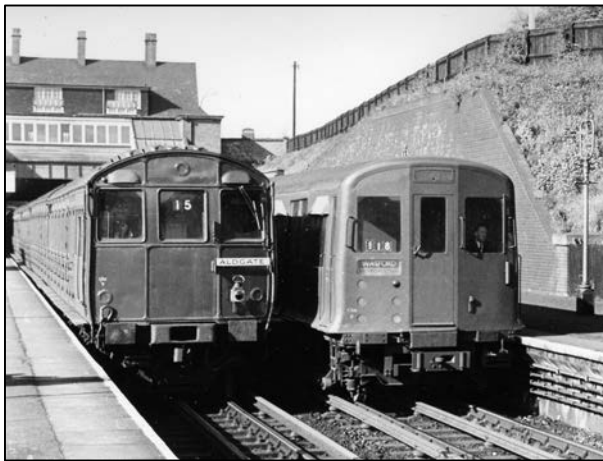
Figure 50: Traditional and modern designs seen at Croxley on the Metropolitan line’s Watford branch about 1961. On the left is a compartment type T Stock train of a design originally dating back to 1910 while, on the right is a P Stock train, introduced in the late 1930s. The flared bodyside skirt of the P Stock was designed to replace the footboard of the older designs but to retain a cover over the gap between the train floor and the platform edge. Collection: B.R. Hardy.
