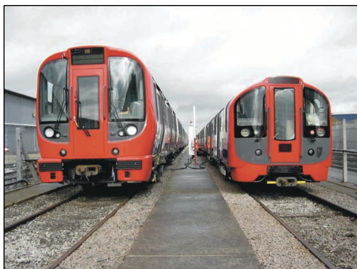
Figure 3: Tube and Surface stock on test at the Bombardier factory in Derby. The smaller train on the right is 2009 Tube Stock for the Victoria line, while the larger train is the S (sub-surface) Stock. The tube car floor is about 300 mm lower than that of the sub-surface stock car and the roof is 800 mm lower. A surviving tradition on the Underground is to identify Sub-surface Stock
