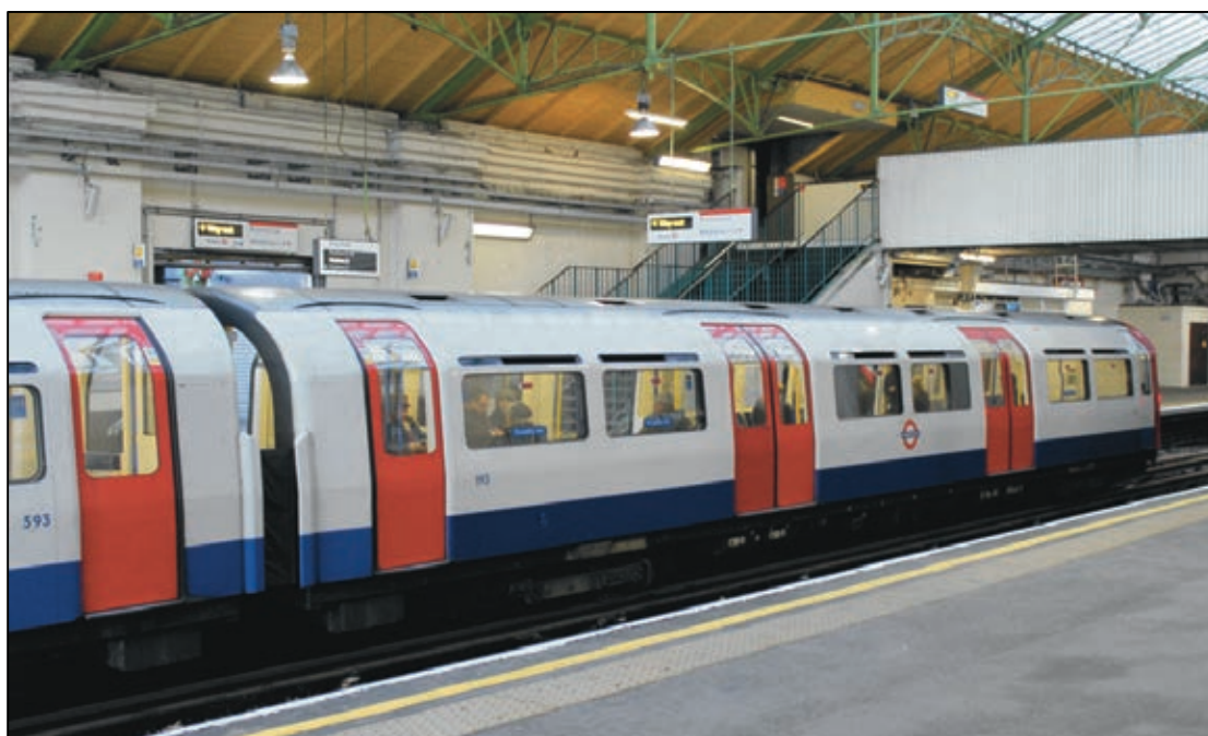
Figure 45: A Piccadilly Line 1973 Tube Stock car, showing the extended tapered car ends that allow longer cars round the tight curves in tube tunnels. This train is at Ealing Broadway (District), working a special service in connection with engineering works in December 2013. Photo: Kim Rennie.
