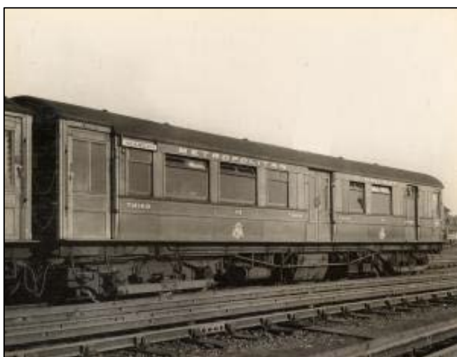
Figure 48: Metropolitan Railway driving motor car introduced in 1913 as seen at Neasden in March 1934. Note the centre doors. These cars were equipped with two sets of traction equipment and four traction motors. They were powerful enough to allow an 8-car train to operate with only two motor cars, one at each end. The Metropolitan never normally ran trains with more than two motor cars. Photo: LT Museum.
