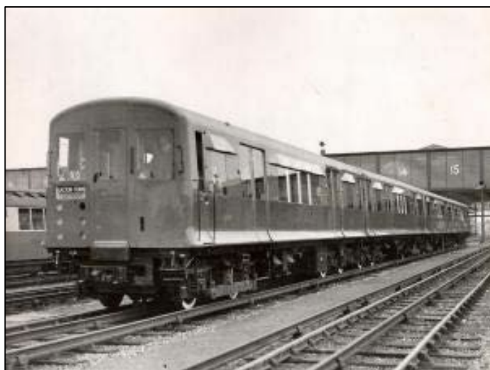
Figure 32: A 4-car O Stock train of 1937 standing at the 'Boston End' of Northfields depot. This was the first Underground stock to have mercury retarder control of braking. It was also fitted with a new system of traction control known as a 'Metadyne', which provided a facility for regenerating braking current into the power supply. Photo: LT Museum.
