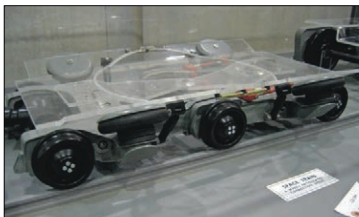
Figure 73: The bogie for the Space Train was a novel, flexible-framed structure with the outer axles driven through cardan shafts by body mounted motors. The centre axle was unpowered. The secondary suspension units were mounted outside the bogie frame and angled
