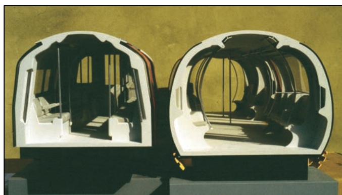
Figure 53: A photo of two models to compare the cross sections of (left) a 1996 Tube Stock car and (right) the Space Train. The body of the Space Train was 218 mm wider than the 1996 Tube Stock. Photo: London Underground.
