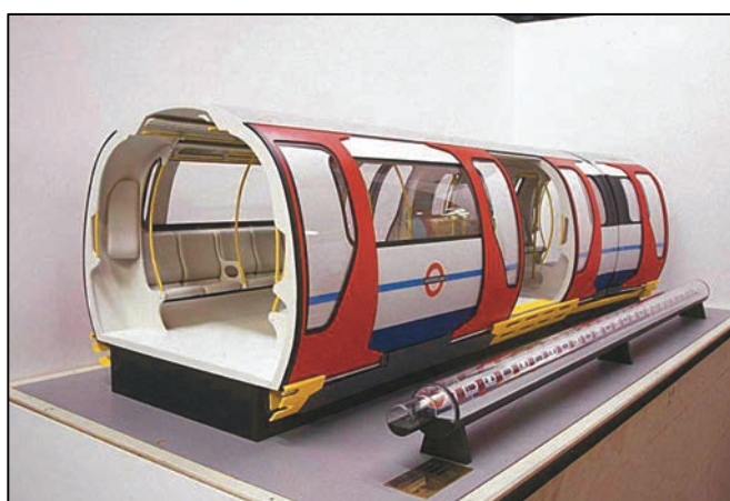
Figure 52: Model of the Underground's Space Train concept. The idea was to widen the car body shape to match more closely the tunnel diameter. Car bodies were to be articulated with wide car connections. There was also an idea that the positive current collection would be at roof level and the return through the running rails. Photo: London Underground.
