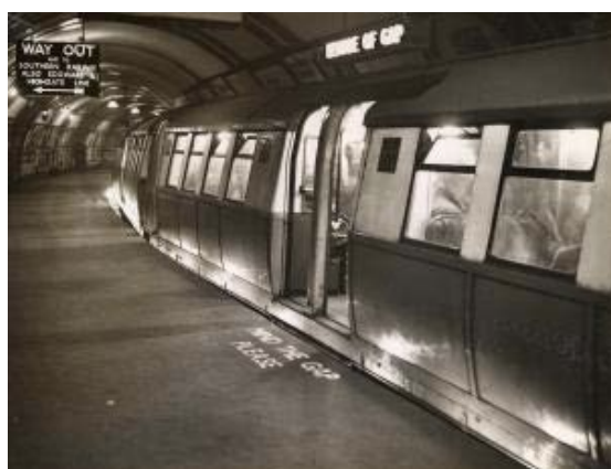
Figure 40: A Bakerloo train at the northbound platform at Waterloo in 1936. The car in the foreground is one of the batch of 40 cars built by Cammell Laird in 1920. The view shows the extreme platform curve at this station. Exhortations to “Mind The Gap” are nothing new (expect perhaps the additional word “Please”) and an illuminated ‘Beware of Gap’ sign hanging from the platform ceiling is also designed to
