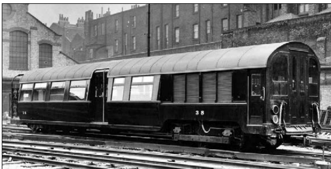
Figure 37: One of two Leeds Forge-built motor cars delivered to the Bakerloo in 1915, seen here in the yard at London Road depot. The car has several new developments in its design. The clerestory roof has been replaced by an arched roof to reduce complaints of the cold in winter; a 3'-2" wide opening has been cut into the car body to allow a centre entrance doorway and the traction control has automatic acceleration. Photo: LT Museum.
