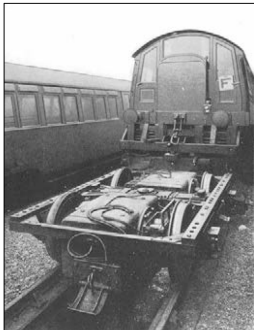
Figure 8: The motor bogie of a W&C motor car with the cab end of a motor car immediately behind. The current collector shoe can be seen at the front of the bogie. It was similar in design to that of the C&SLR, being a hinged flap. It was mounted on a wooden block attached to the front of the motor case. The huge motors can be seen occupying most of the space between the wheels. The motor armatures were mounted directly on the axles. Photo: Cassier's Magazine, August 1899, p300.
