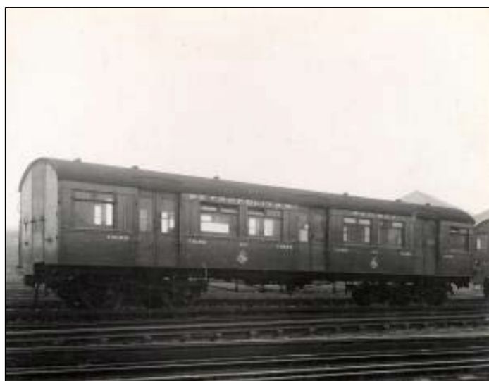
Figure 49: Metropolitan Railway 3 rd Class Saloon Stock trailer car no 103 of 1921, as seen at Neasden in March 1934. Like the contemporary District stock of 1920 (The F Stock), this design had three sets of double doors. After 15 years of operating a high volume urban railway, the Underground companies realised that more doors were needed to keep station dwell times down to a
