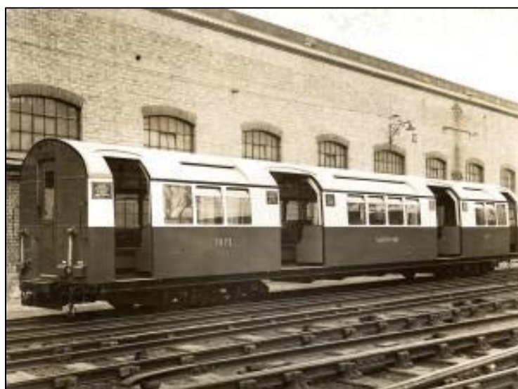
Figure 44: A trailer of Standard Stock built in 1931, seen in new condition at Ealing Common depot. The 1931 and 1934 batches of this stock, built for the Piccadilly Line, were longer than the earlier versions and the trailers had single end doors added. The body ends were slightly tapered to allow the longer cars to negotiate the tight curves on some of the tunnel sections. Photo: LT Museum.
