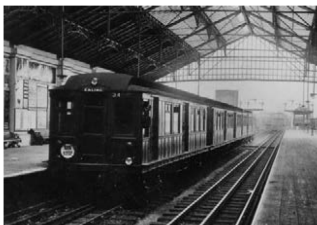
Figure 36: 4-car unit of District Railway 1905 B Stock at Ealing Broadway about 1909 after its conversion to hand-worked doors. This stock was fitted with air powered doors when delivered but these were poorly designed and slammed shut, trapping people and clothing and causing injuries. They had brass edges instead of the rubber edges used today. The conversion to hand operated
