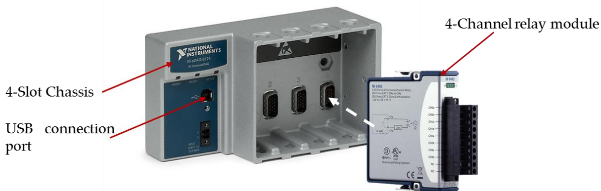
Figure 7-16, National Instruments chassis and relay control board
