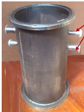
KF ports for water vapour, pressure transducer and thermocouple connections
