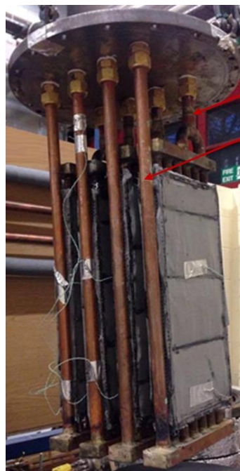
Figure 7-4, Finned tube heat exchangers of the adsorber bed
