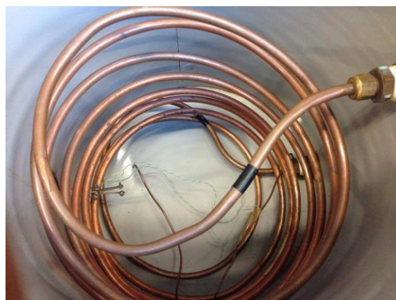
Figure 6-7, Pictorial view for the condenser cooling water helical copper coil
