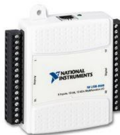
Figure 6-15, National Instruments control board, “NI 6008”
