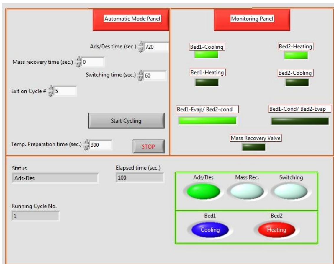
Figure 7-17, User interface of the “Labview” software to control the actuated ball valves
