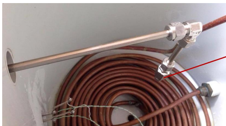
Figure 7-8, Seawater spraying nozzle in the evaporator
