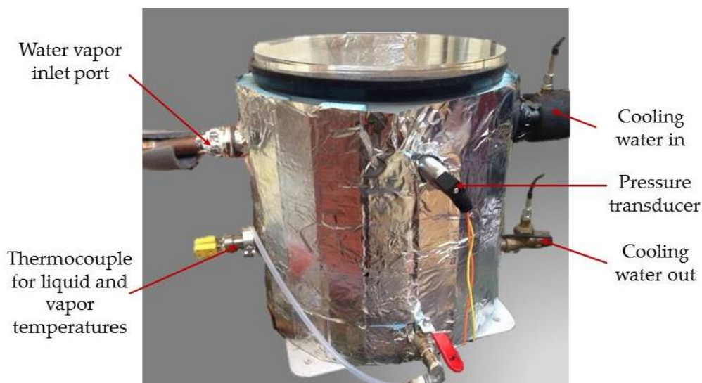
Figure 6-6, Pictorial view for the condenser with different inlet and outlet ports and connections
