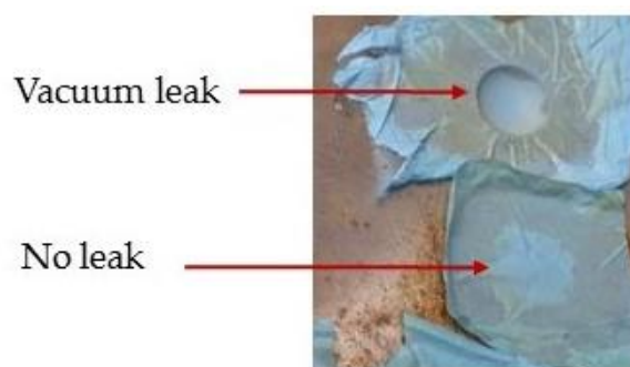
Figure 6-30, Vacuum inspection using the diaphragm technique
