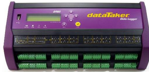
Figure 6-27, Data logger used for logging temperature and pressure readings, “dataTaker DT85”
