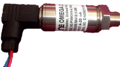
Figure 6-21, Pressure transducer “PXM319-0.35AI”
