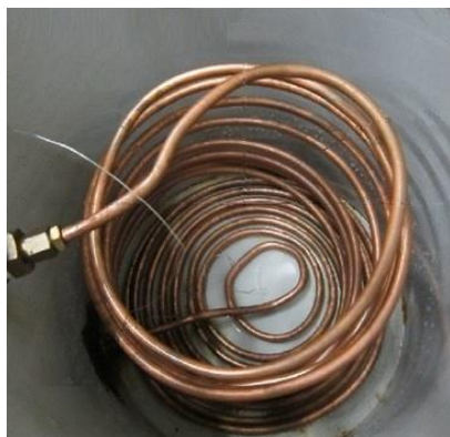
Figure 6-5, Pictorial view for the evaporator chilled water spiral copper coil [12]
