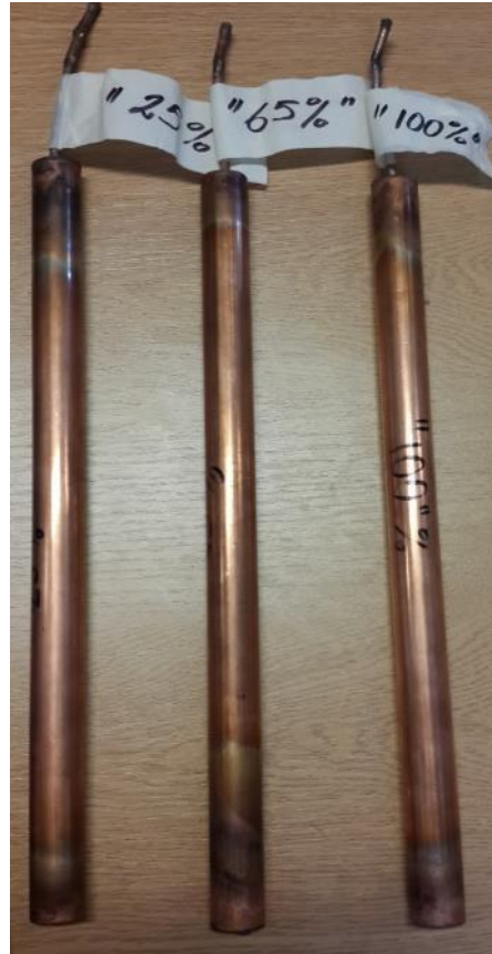
Figure 4.2 Three TPCT with three different fill ratios
