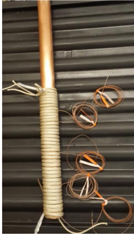
Figure 4.3 heat pipe with AC rope heater
