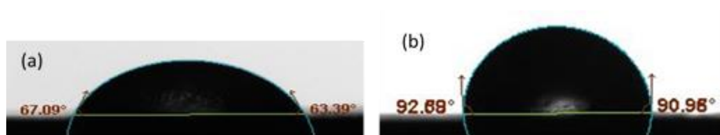
Figure 5.6 Measured contact angle for: (a) Rough and (b) plain copper surfaces [178]
