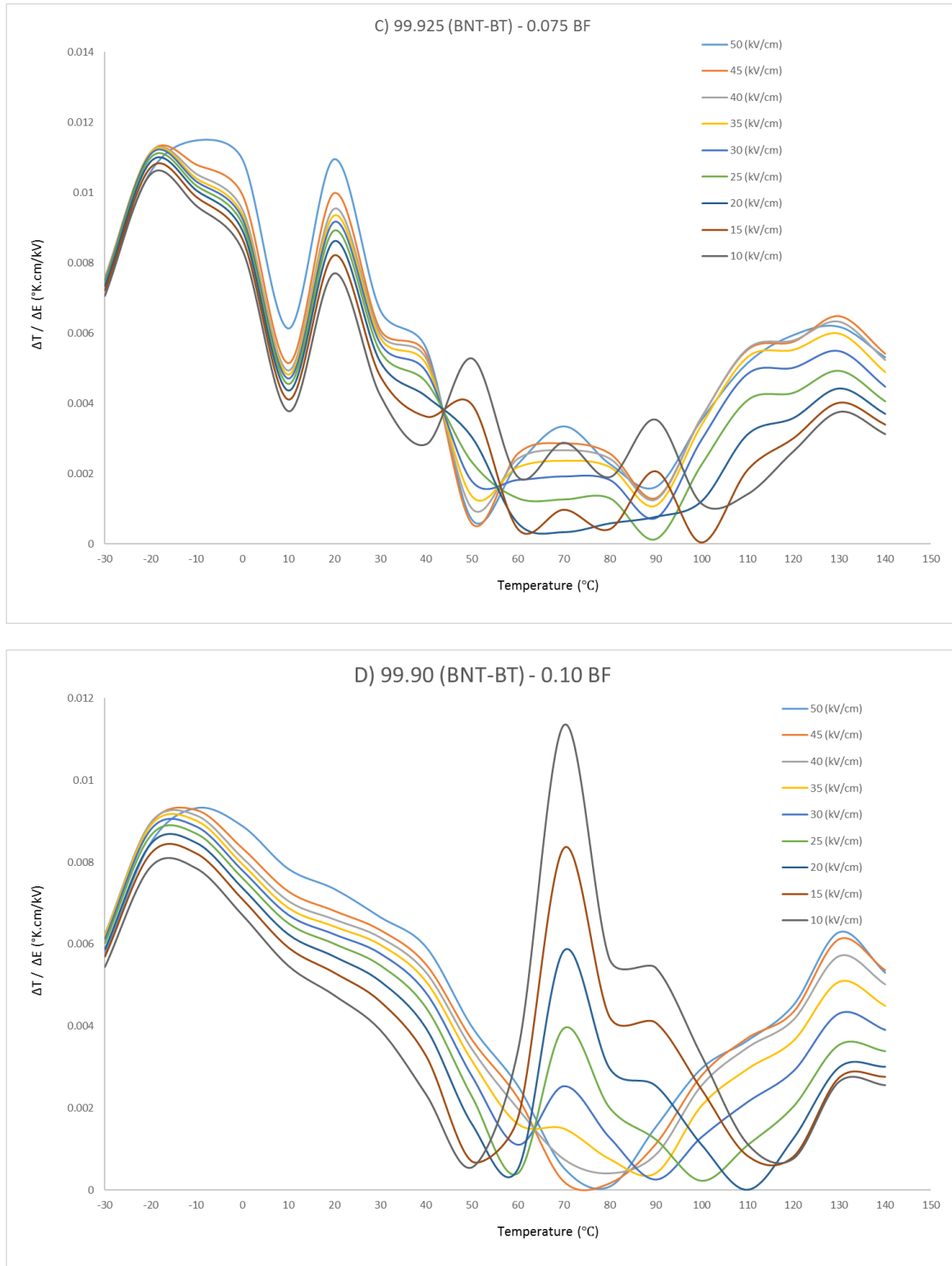
Figure 5-22: The ECE figures of merit of the (1-x) BNT-BT-x BF samples for x A) 0.025, B) 0.05, C) 0.075, and D) 0.1 measured between -30 and 140°C by the indirect method.
