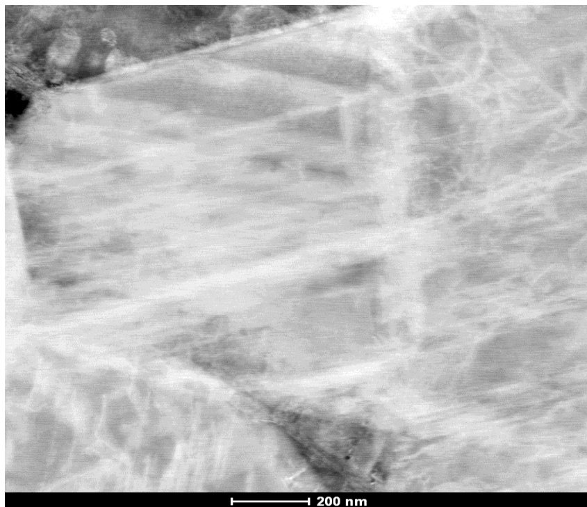
Figure 33. TEM image of sample after treatment. The fracture lines in the tungsten carbide particle is more visible at higher magnification.
