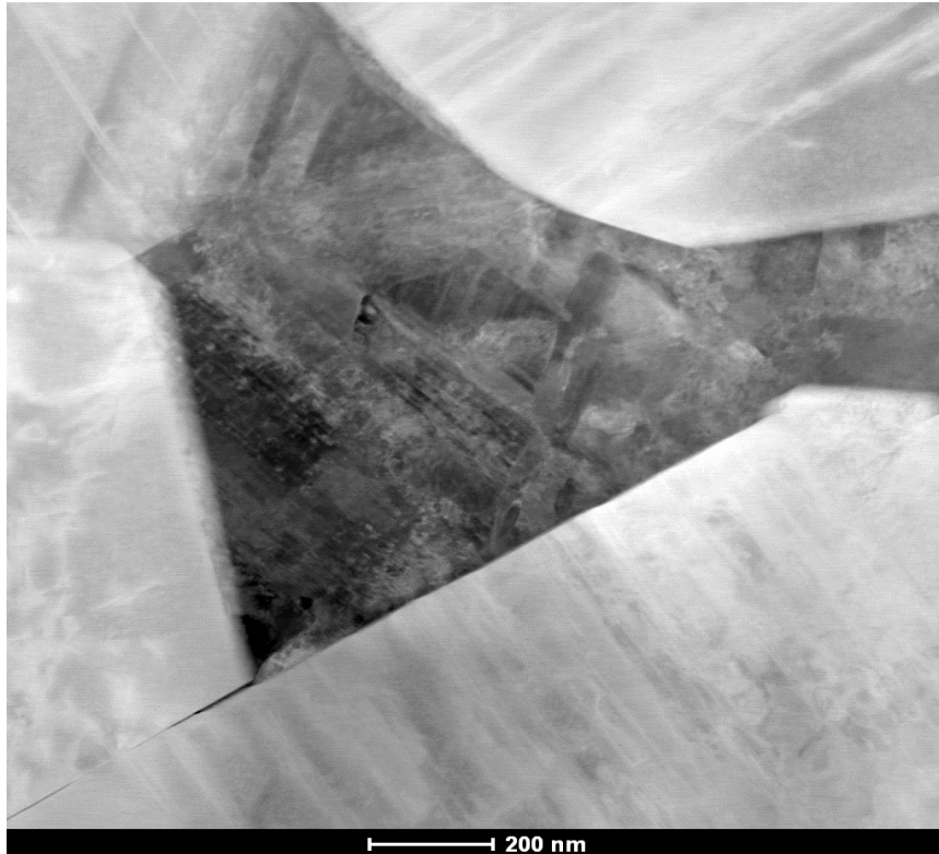
Figure 32. TEM image of sample after treatment. The cobalt binder, surrounded by the tungsten carbide particles, appears to be highly disordered.
