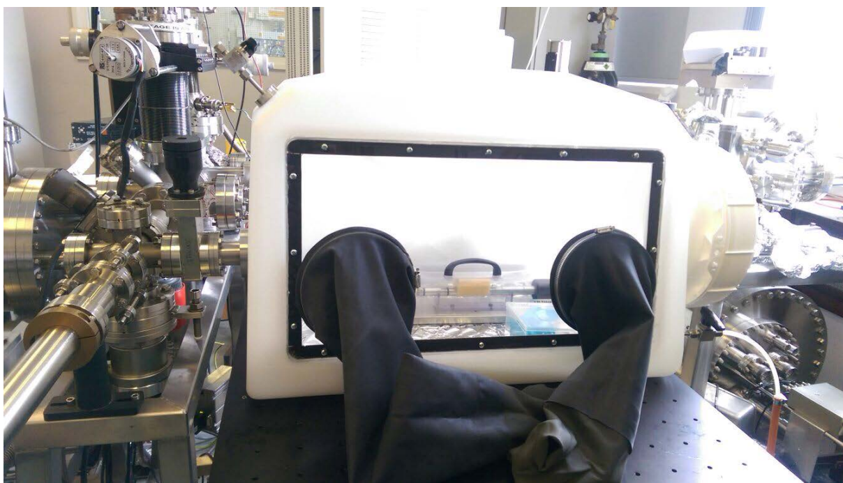
Figure 3.9: A photo of the gas transfer box attached to the cluster source. On the left-hand side the box is connected to the cluster source by a gate valve. On the right-hand side there is the large opening for inserting and removing the STEM arm. The gas inlet and outlet can be seen at the top left and bottom right corners of the box.
