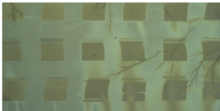
Figure 4.34: Discharge during exposure at 100 keV with 2nA.
