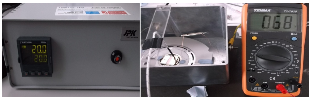
Figure 3.14: When the heater read 20 °C, the thermocouple read 68 °F = 20 °C
