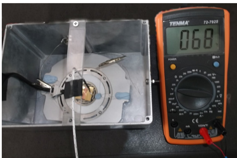
Figure 2.27: The heater with token inside a Faraday cage and a thermocouple on top of the token's surface.
