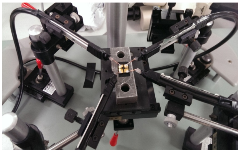
Figure 3.10: Experimental setup with copper probes with silver paint
