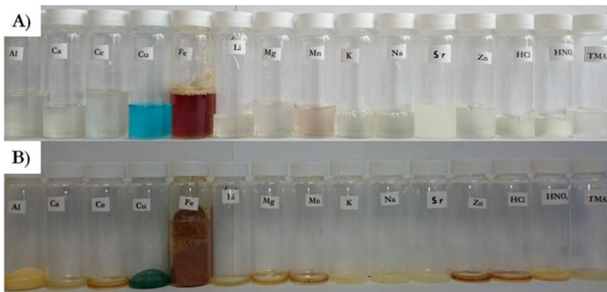
Figure 2.2 Gelatin with various metal nitrates before (A) and after (B) drying at 70 °C
