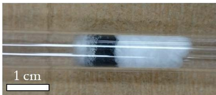
Figure 4.2 Sample packed ready to be placed into reactor
