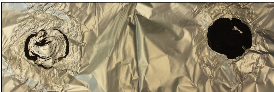
Figure 4.5: GO multilayer membrane after HP with each external layer of Nafion stuck on the aluminium foil.
