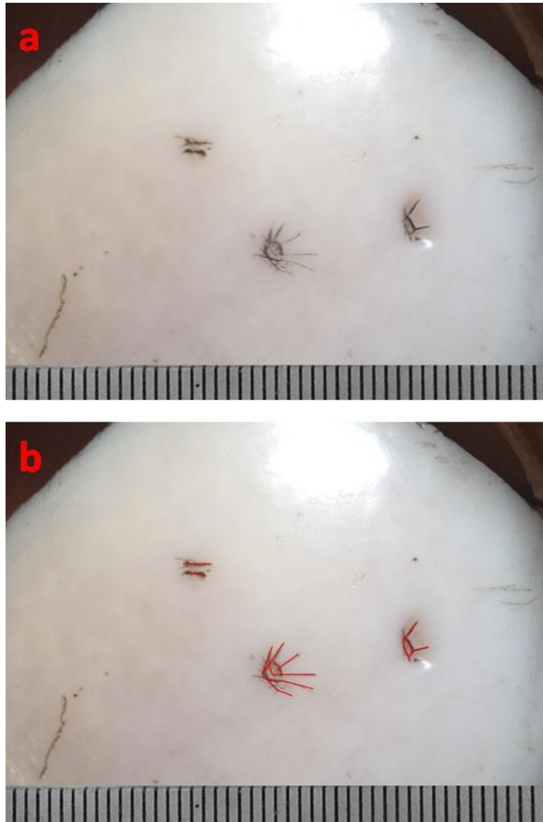
Figure 3.17. Total crack length (a) Cartilage surface cracks highlighted with the aid of India ink. (b) Red lines were drawn along the surface cracks to highlight damaged areas.
