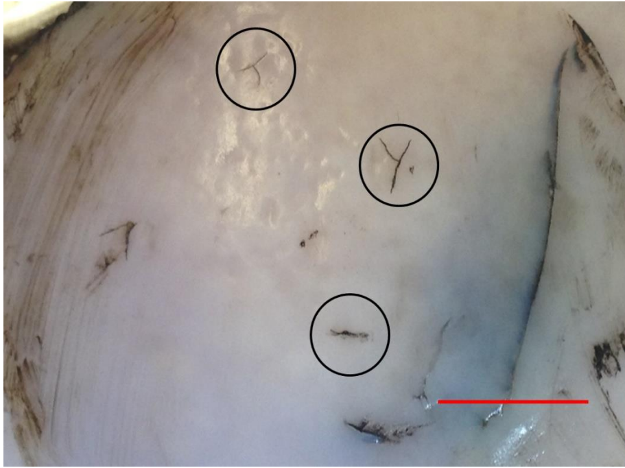
Figure 3.7. Three sites were chosen on a cartilage-on-bone specimen to perform compression tests. The cartilage surface damage was highlighted with the aid of India ink. Cracks appeared on the cartilage surface following testing. Black circles inserted in the image are 5.2 mm in diameter, the same diameter as the indenter. Scale bar (red bar at the bottom right) ~ 1 cm.
