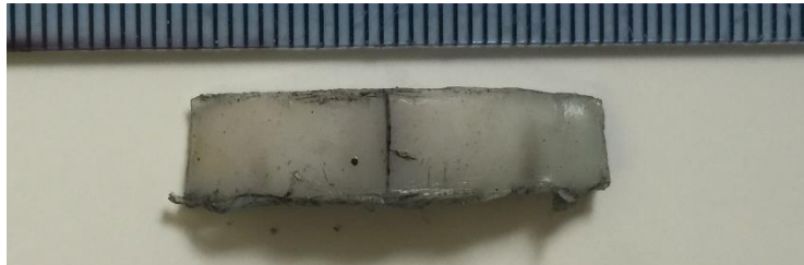
Figure 4.7. An initial crack of 0.5 mm depth was cut into the centre of the cartilage-on-bone specimen.
