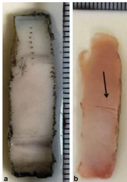
Figure 4.16. Cartilage surface crack observed on specimens that reached run-out at loading frequencies of 1 Hz and 10 Hz (a) Top view of the selected specimens after run-out was reached at a loading frequency of 1 Hz and (b) 10 Hz. Both specimens in these images were loaded between 6-60 N.
