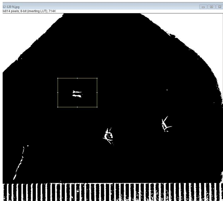
Figure 3.15. The area of damage was identified at each individual test site as shown by the rectangular box.
