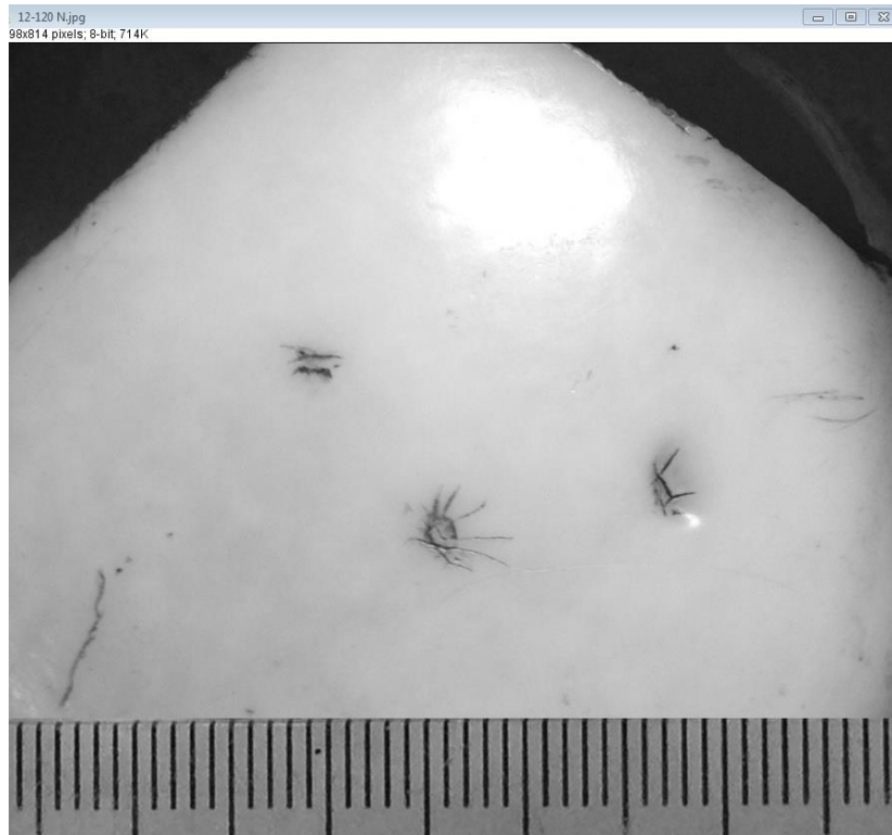
Figure 3.12. An example of a gray-scale image. Images were converted into 8-bit grayscale before the application of threshold.
