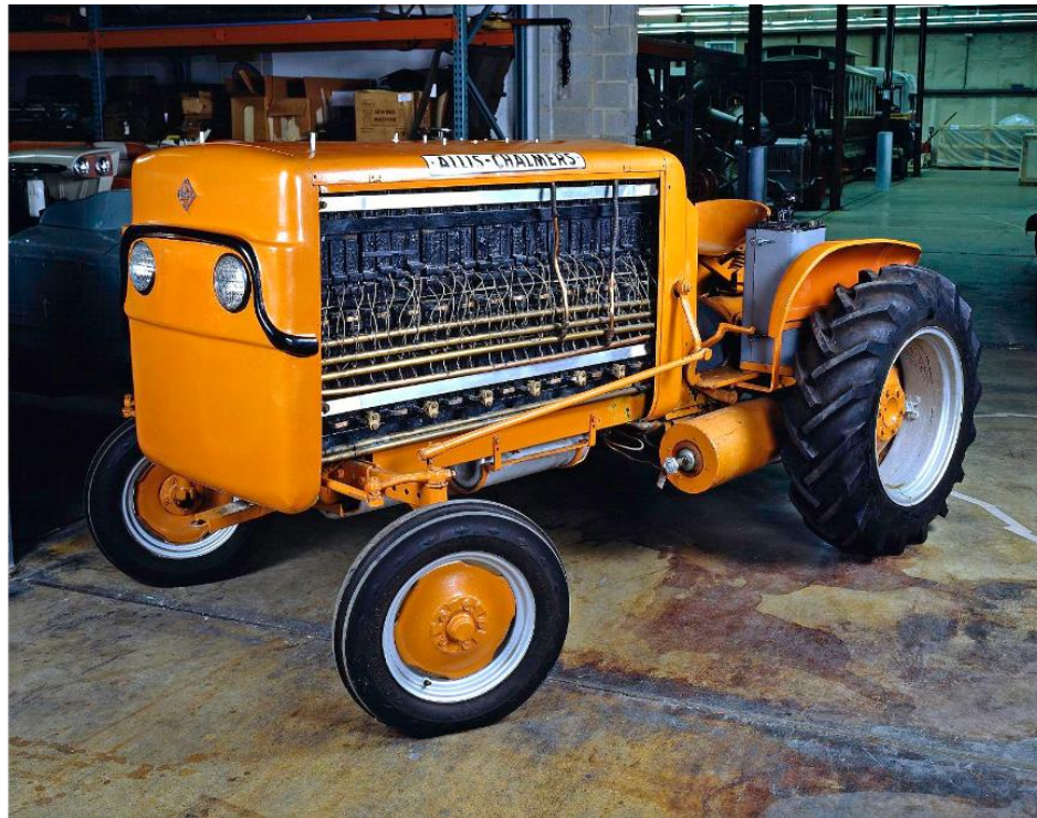
Figure 1.2 – The first fuel cell vehicle the Allis-Chalmers Fuel cell Tractor, 1959. Reused under the fair use policy from the National Museum of American History website 29
