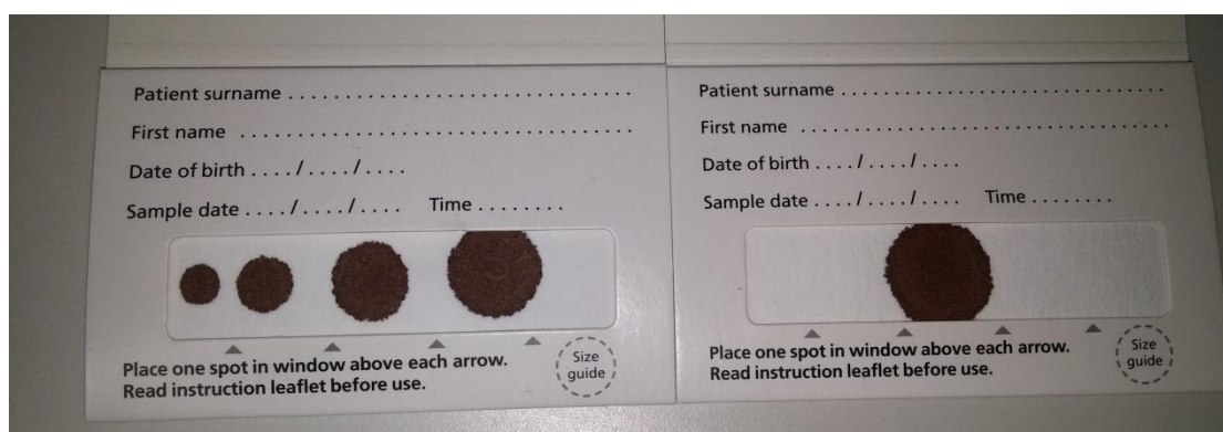
Figure 3.5 – DBS created using different volumes of blood. From left to right: 10 µL, 20 µL, 50 µL, 75 µL and 100 µL.
