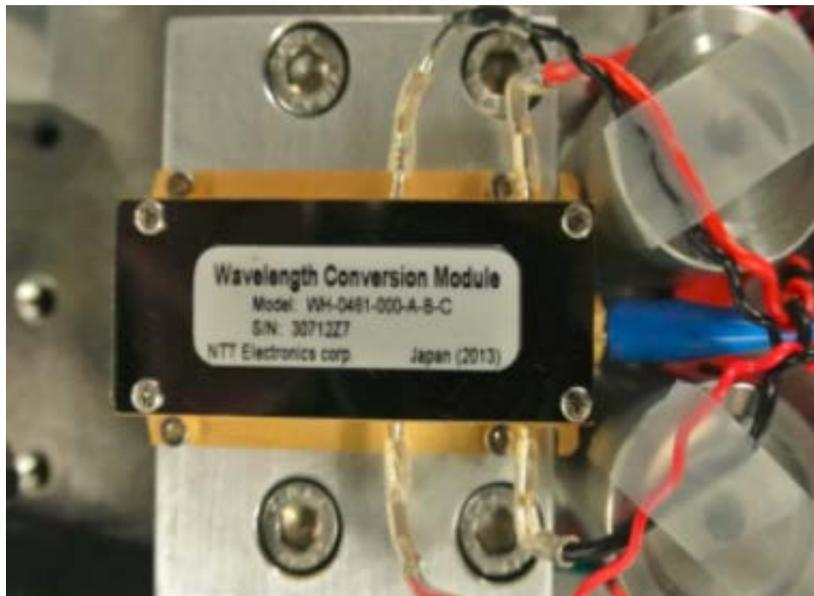
Figure 3.6: The wavelength conversion module is mounted on a customized aluminium base.
