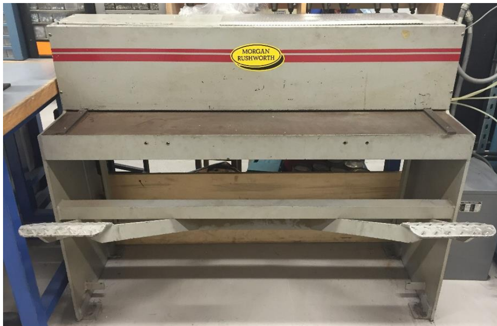
Figure 3.1-2 MORGAN RUSHWORTH shearing machine used to cut AA6082 as-received sheets.
