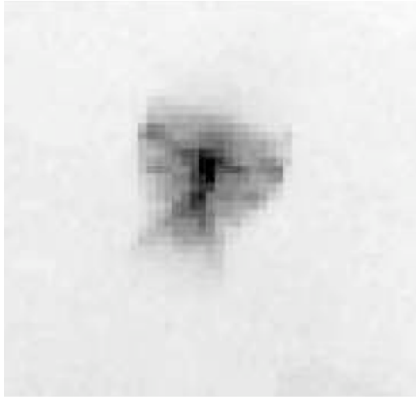
Figure 4.2: A high resolution of the usual SMEI PSF. The image of an unresolved point object is smeared over around 250 pixels. This image is a 50 \times 50 pixel cut from an engineering mode frame in which the image is unbinned. Images are typically binned by a factor of 4 \times 4 to generate science frames.
