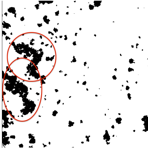
Figure 4.9: High-speed camera recorded images of coffee particles from \Psi_B . Circled particles most likely correspond to aggregates of material not properly dispersed
