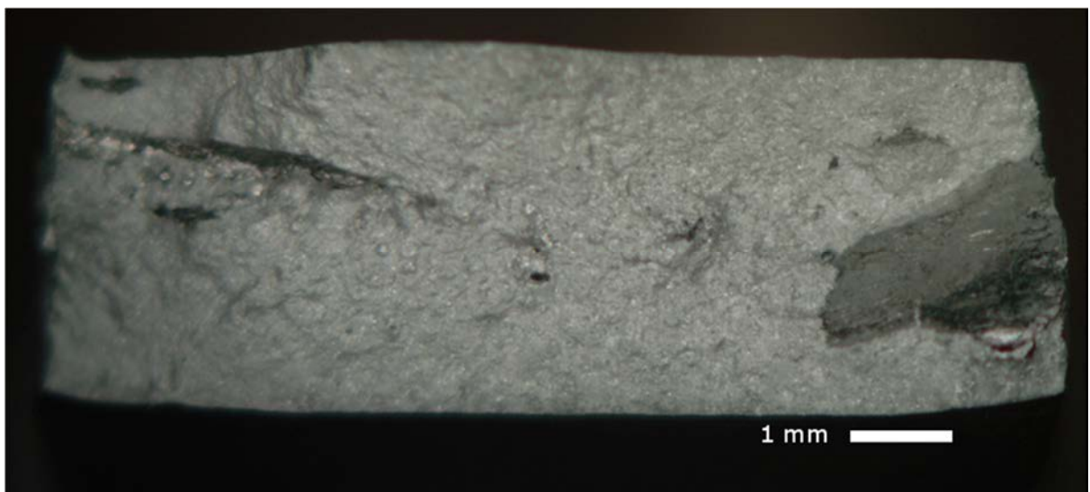
Figure 10-38: Optical image showing a shiny planar defect on the right hand edge of the test bar.
