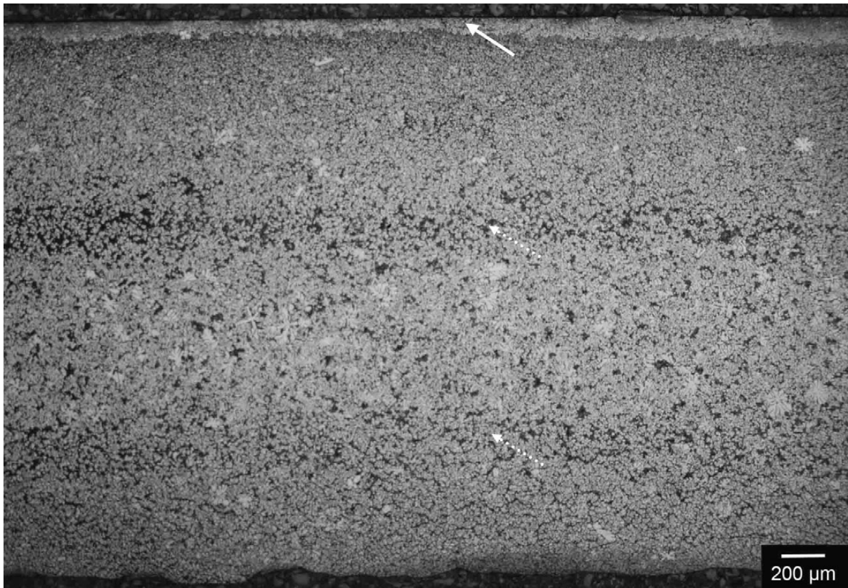
Figure 2-3: Typical HPDC microstructure showing distinct banding, from Otarawanna et al. [30]
