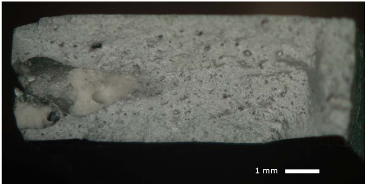
Figure 10-54: An optical image showing the inclusion towards the left of the image, together with some pores on the order of 100 \mu\text{m} in size.
