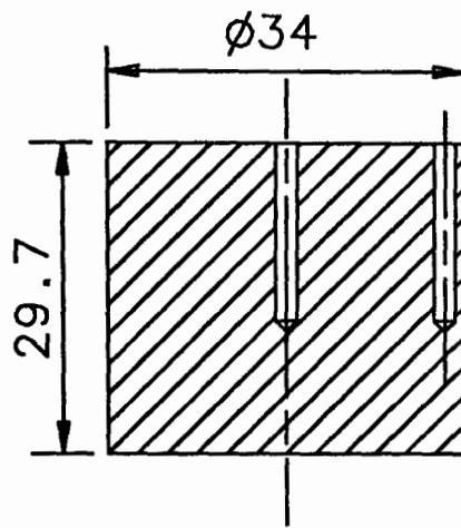
Fig. A.1 Billet used for experimental calibration curves
