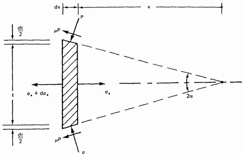
Fig. 2.5 State of stresses in the slab method for simple plane-strain [34].
