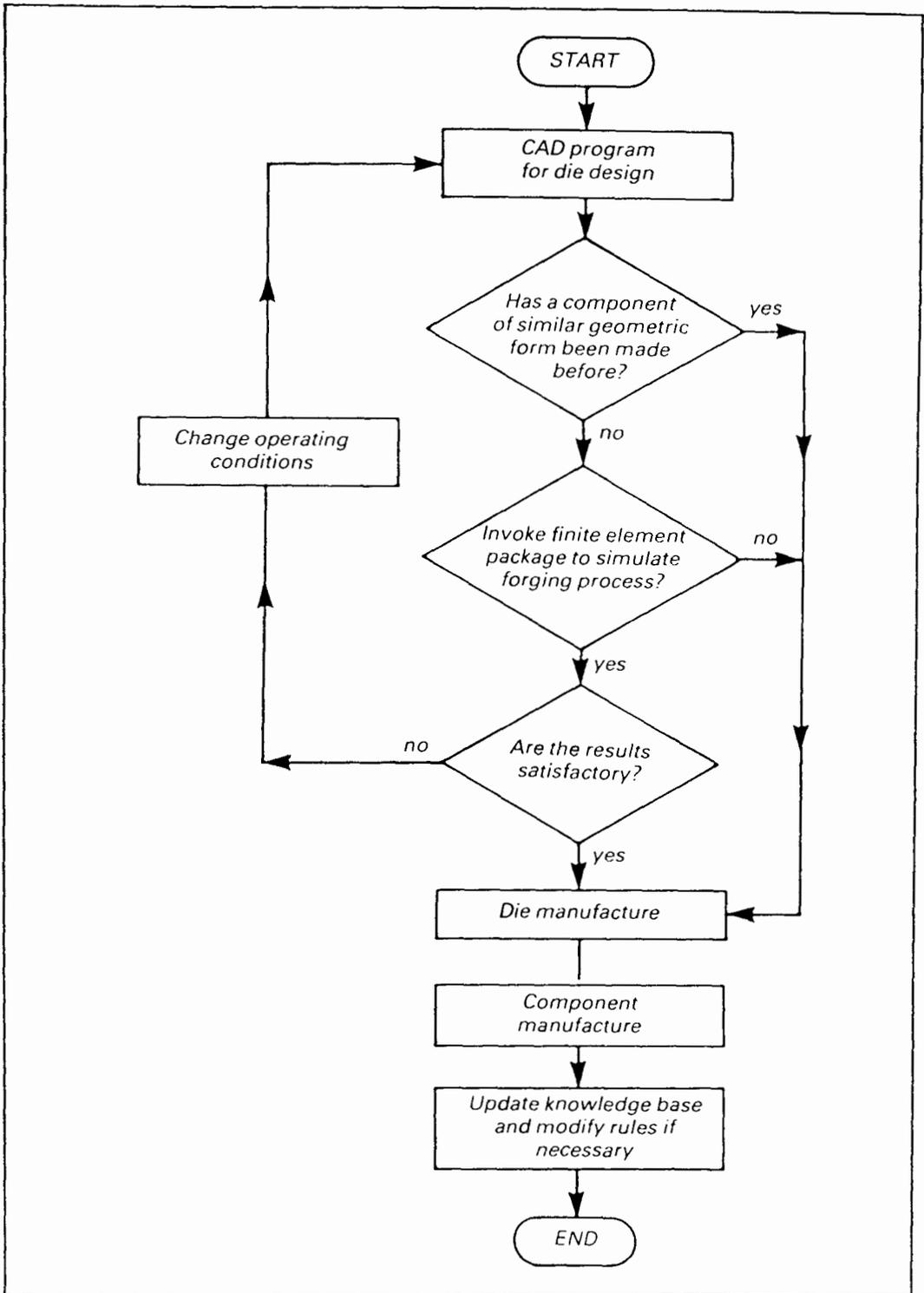
Fig. 2.14 A brief illustration of a forging Expert System [86], [87] and [88].
