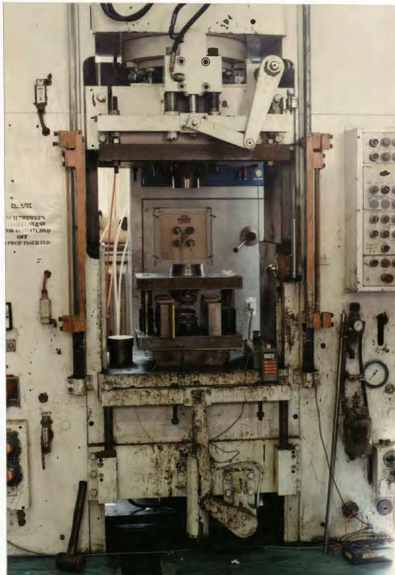
**Fig. C.5 The 1500 KN hydraulic press used in the experiments.**
