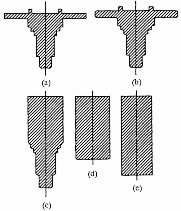
Fig. 2 The operational sequences for a Stub Axle
