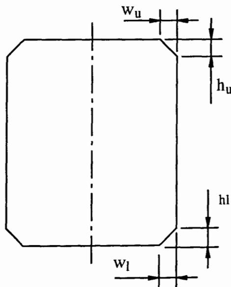
Fig. 5.2 Schematic illustration of a deformed billet in closed–die upsetting.
