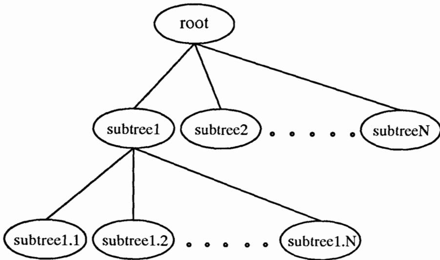
Fig. 6.2 The general representation of a tree-type data structure (frame-based representation) [59].
