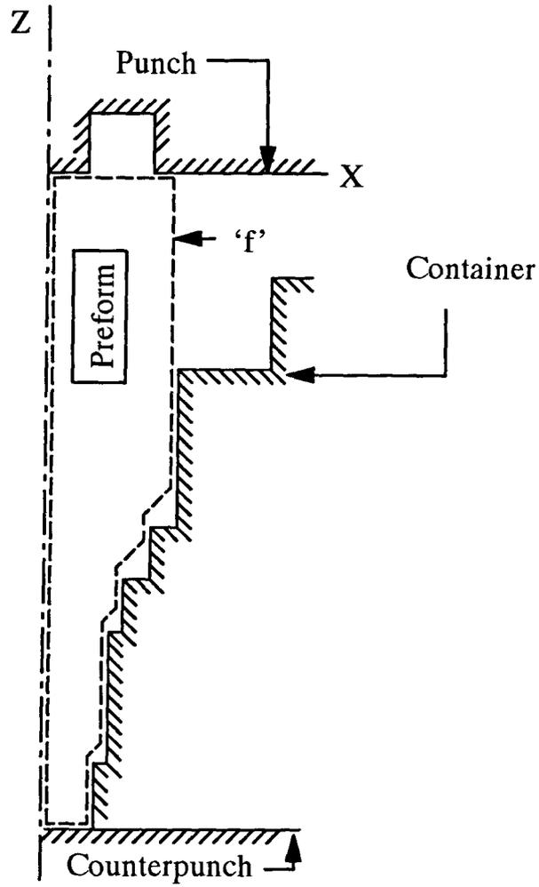
Fig. 4.15.b Schematic illustration of producing 'finish' from 'preform' (upper and lower dies)
