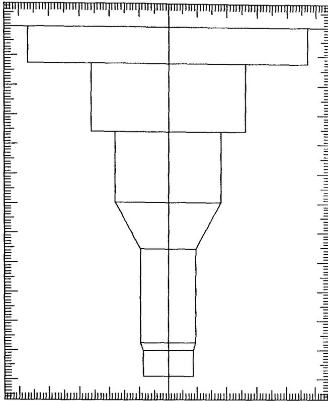
Fig. 8.3 Maestro Stub Axle, WFM 2029 (machined part)
