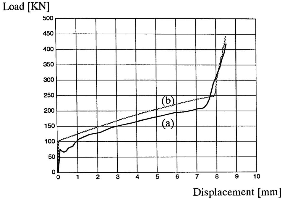
Fig. 7.13 Load–displacement curve obtained from experiment and simulation
