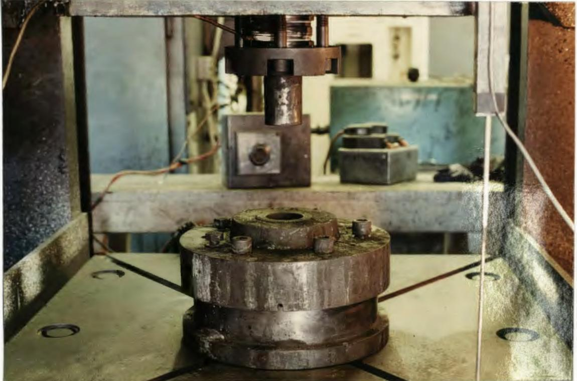
**Fig. C.3** The tool sets used in the experiments.
