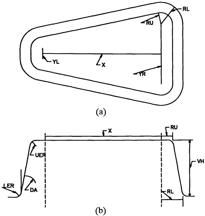
Fig. 3.1 The general definition of CONE (positive primitive) [92]
