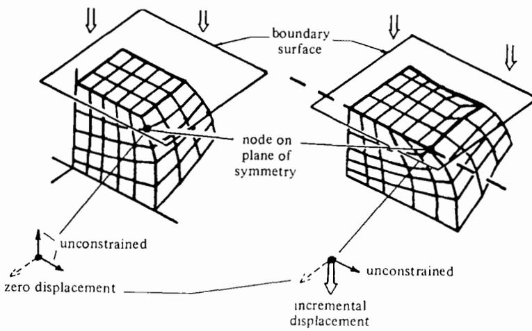
Fig. 4.6 Contact of a boundary surface with a node subject to previous constraining condition [52]
