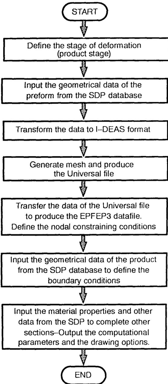
Fig. 3 The process of producing the EPFEP3 datafile.
