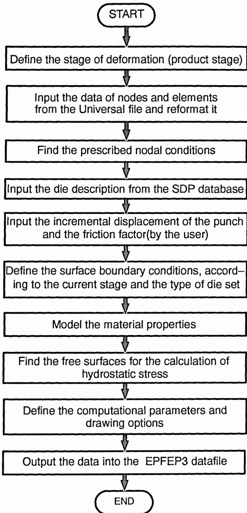
Fig. 4.12 The main actions of producing the datafile
