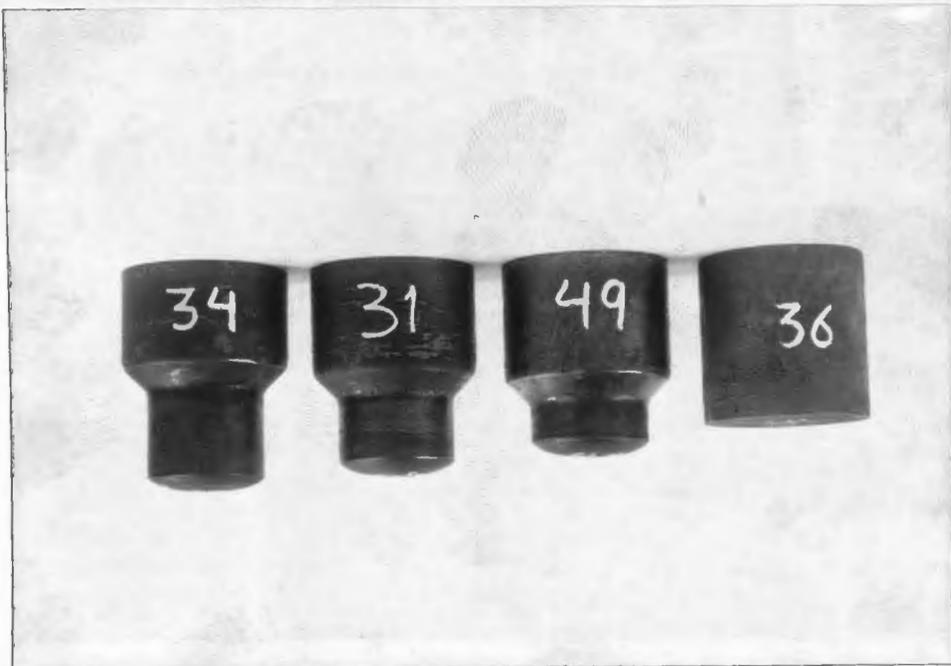
**Fig. C.2** The geometry of the specimens in forward extrusion
