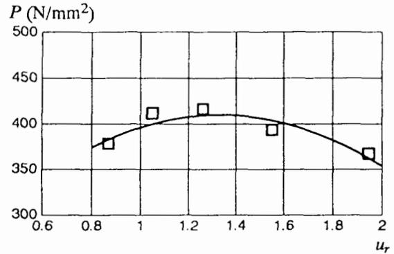
Fig. 6 Variation of average pressure with upset ratio for 2% unfilled die cavity (cheese diameter=41 mm)
