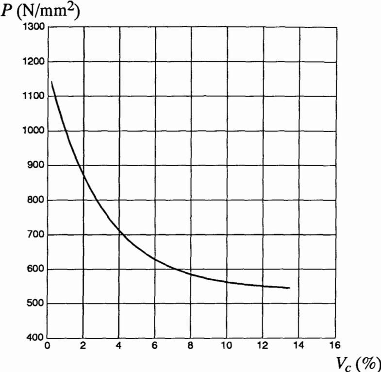
Fig. 5.5 Variation of average pressure  $P$  with unfilled corner volume  $V_c$  (test No. 1) –Fitted equation:  $P(V_c)=539+645.5e^{-0.326V_c}$
