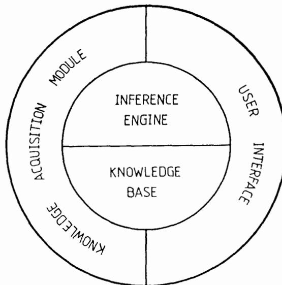
Fig. 2.11 A schematic illustration of different components of an Expert System [61].
