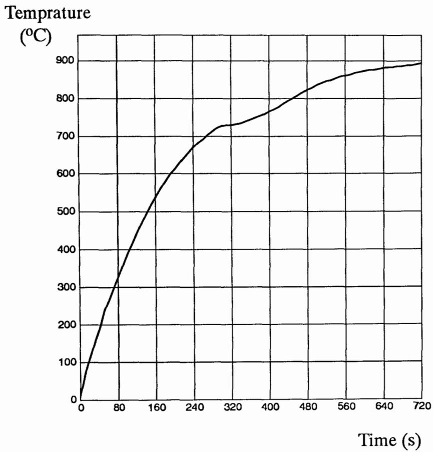
Fig. A.2 Heating curve for the centre of the billet
