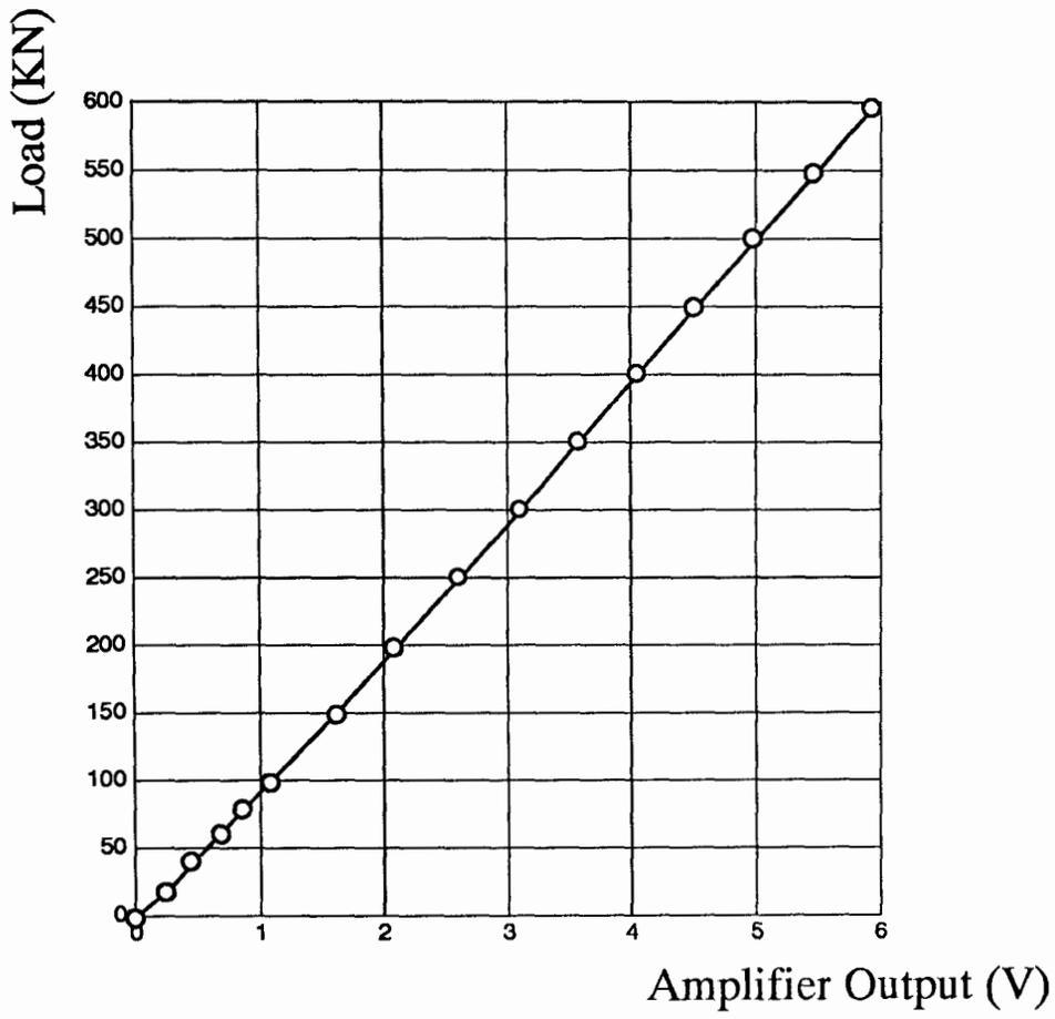
Fig. A.10 Load-cell calibration curve
