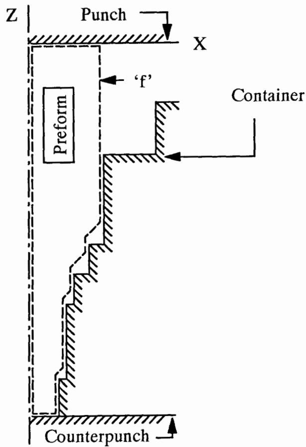
Fig. 4.15.a Schematic illustration of producing 'finish' from 'preform' (flat punch)
