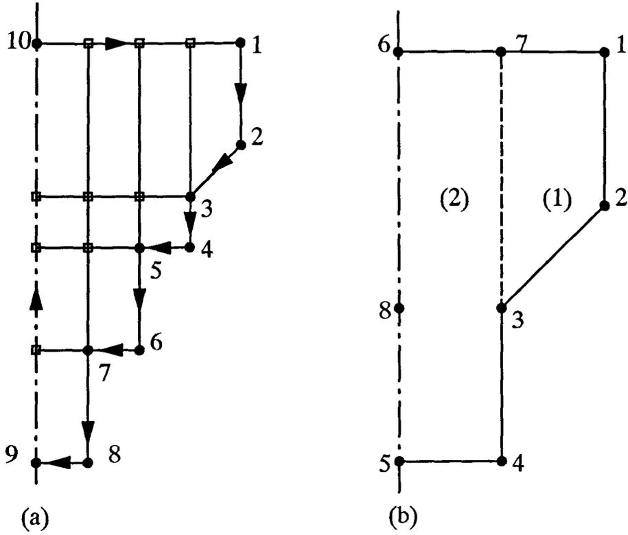
Fig. 4.11 Dividing the half cross-section of 'preform' to sub-areas to produce Mapped mesh
