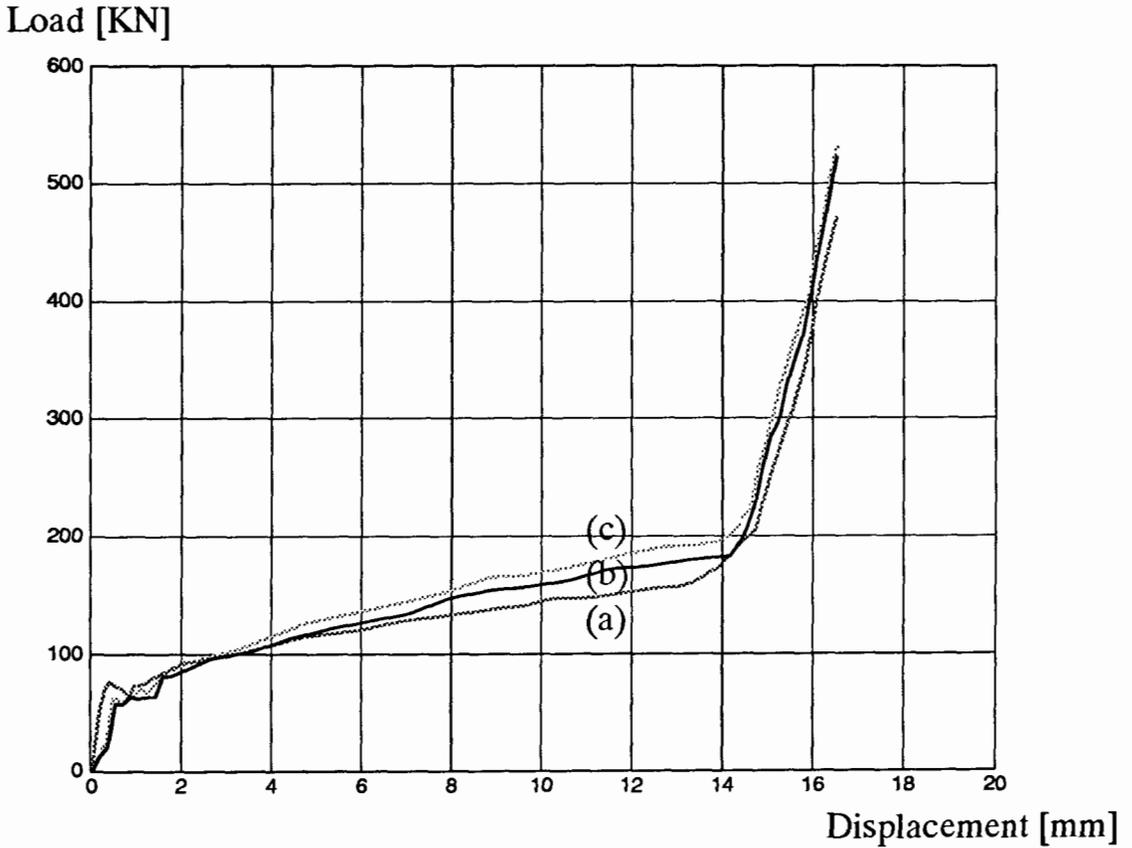
Fig. 5.8 The effect of lubrication condition on forging load in closed-die upsetting
