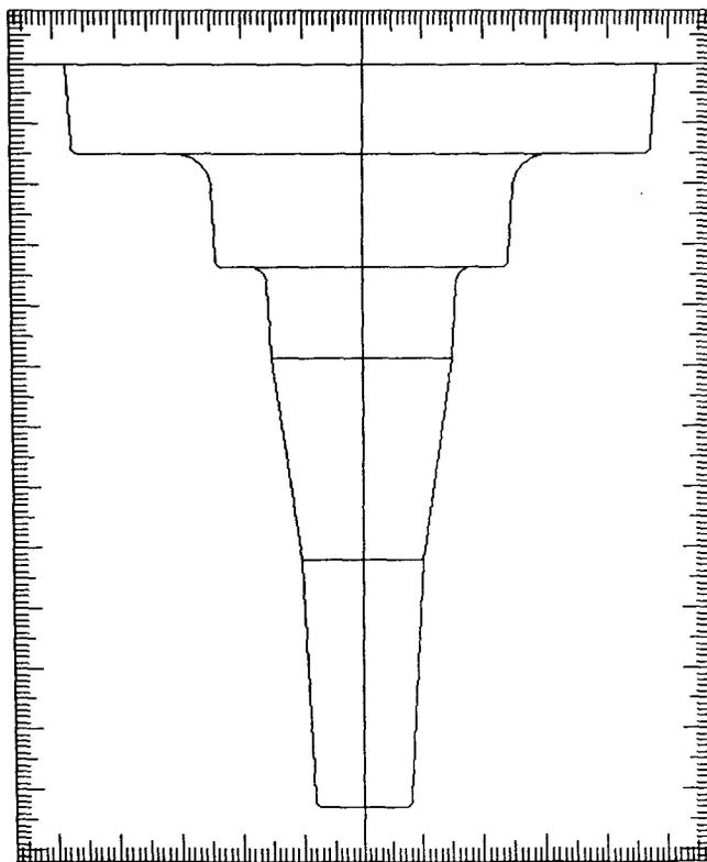
Fig. 8.4 Stub Shaft Forging, WFM 2023 (machined part)
