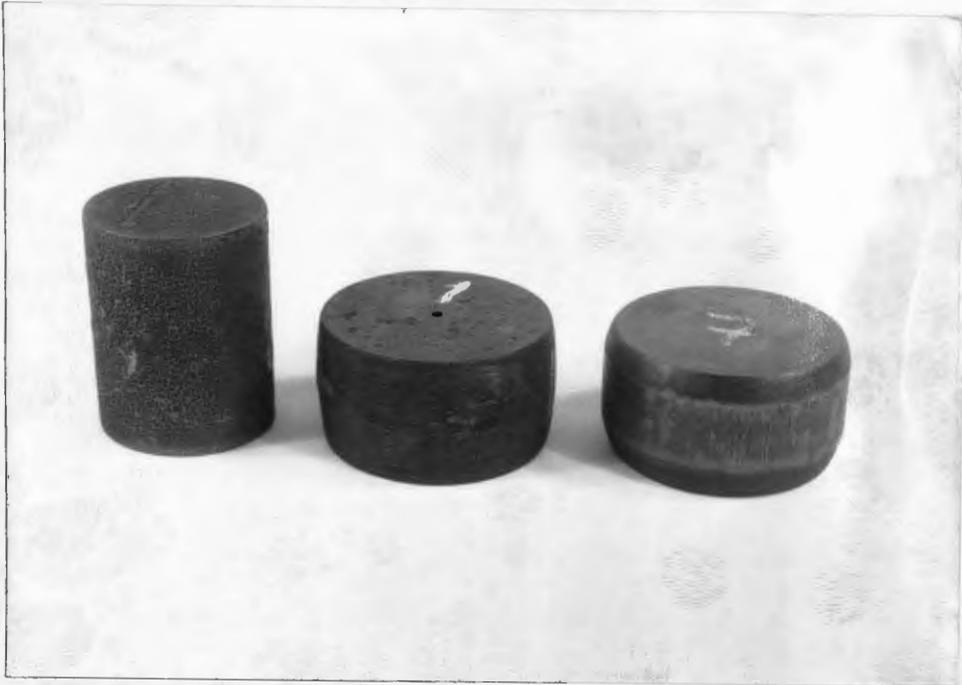
**Fig. C.1** The geometry of the specimens in closed-die upsetting
