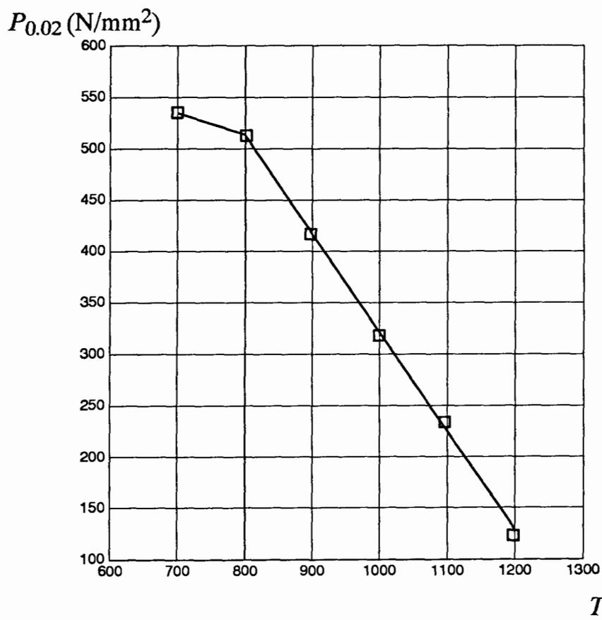
Fig. 5.9 Variation of average pressure at 2% unfilled die cavity ( $P_{0.02}$ ) with billet pre-heat temperature  $T$  for closed-die upsetting- test No. 5.
