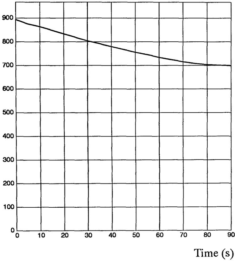
Fig. A. 3 Cooling curve for near the surface of the billet
