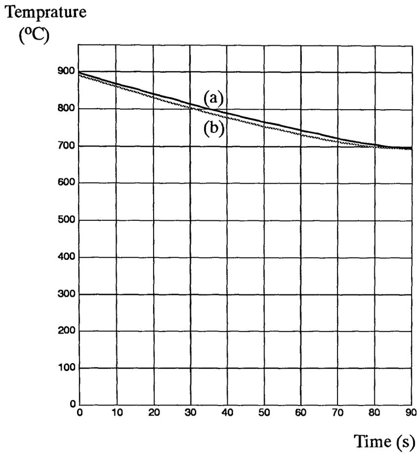
Fig. A.9 Cooling curves near the surfaces of two examples with two different lubricants (example No. 3 in table 5.1)
