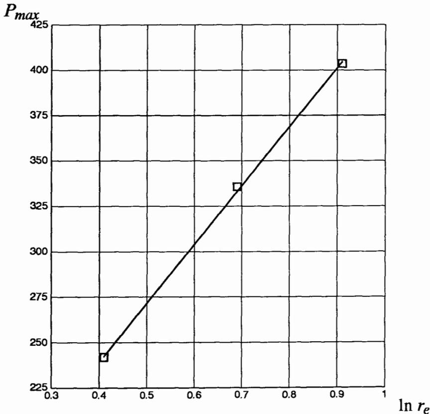
Fig. 5.12 Variation of maximum average pressure  $P_{max}$  with extrusion ratio  $r_e$  for forward extrusion— test No. 8.
