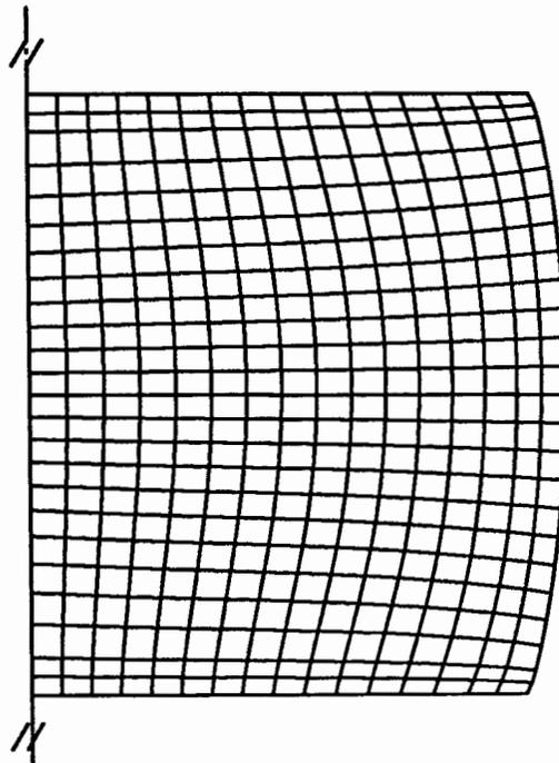
Fig. 7.10 The geometry of the deformed mesh corresponding to the stage in Fig. 7.9
