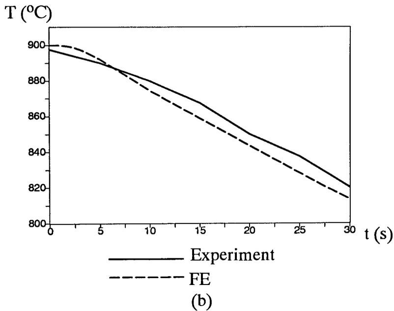
Fig. 7.5 Variation of billet temperature with time (transfer period)
