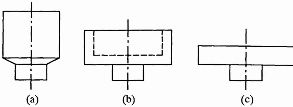
Fig. 2.3 Some operational sequences in forging [11].
