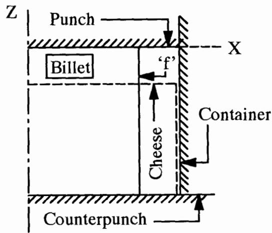
Fig. 4.13 Schematic illustration of producing 'cheese' from 'billet'
