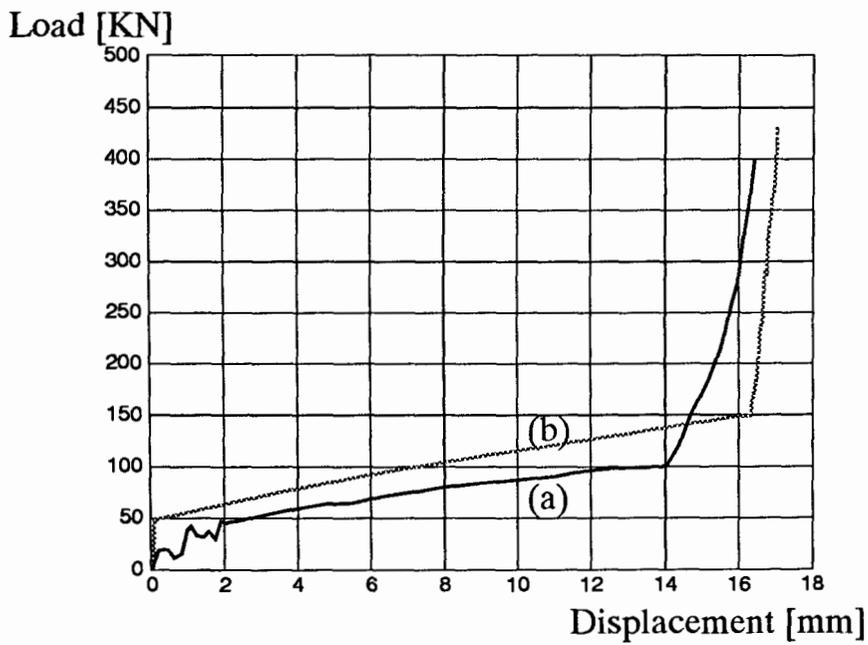
Fig. 8.10 Load–displacement curves obtained from experiment and simulation corresponding to Fig. 8.9.
