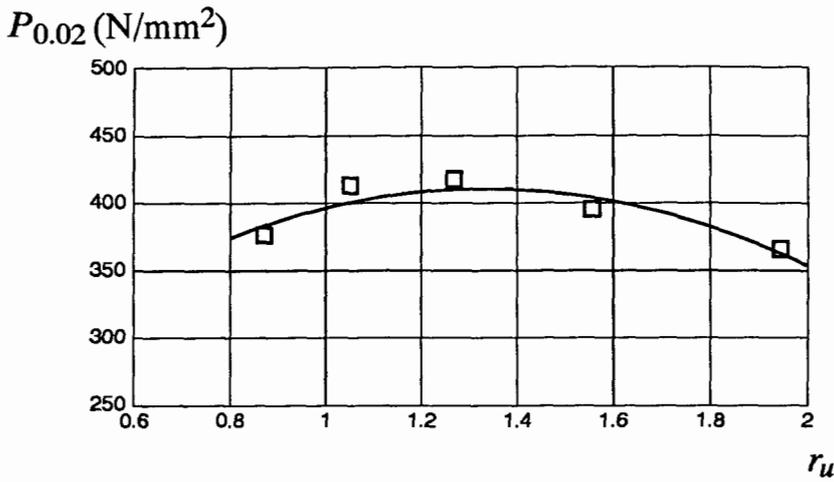
Fig. 5.6 Variation of average pressure at 2% unfilled die cavity ( $P_{0.02}$ ) with upset ratio  $r_u$  for closed–die upsetting–test No. 2
