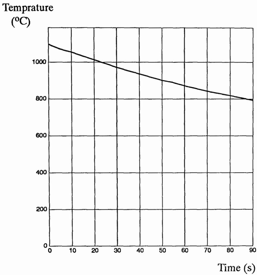
Fig. A.7 Cooling curve for near the surface of the billet
