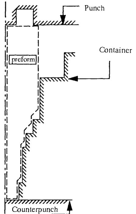
Fig. 4 Schematic illustration of producing the 'finished' part from the 'preform'.
