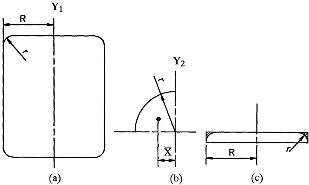
Fig. B.1 Schematic illustration of cheese-die geometry
