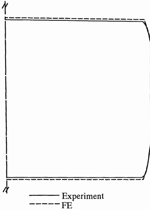
Fig. 7.11 Comparison between the geometry of the workpiece and that of the mesh, in the stage of corner filling (scale=4:1)
