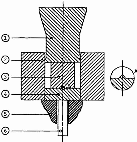
Fig. 5 Schematic illustration of the die-sets of closed-die upsetting (producing the 'cheese' from the 'billet')
