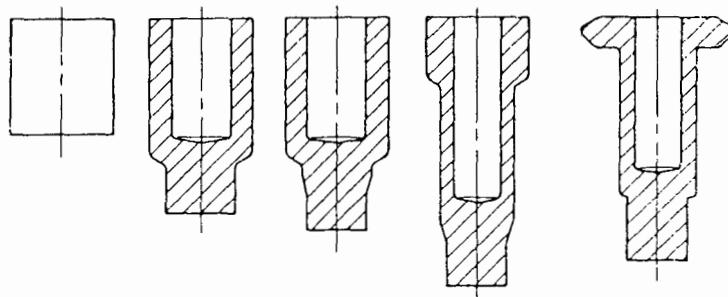
Fig. 2.4 Schematic illustration of operational sequences for a gear blank [4].
