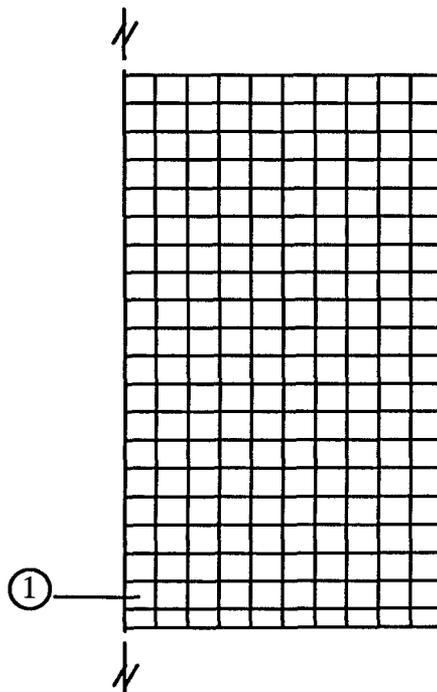
Fig. 7.7 FE mesh used to obtain cooling curves by the simulation corresponding to Fig. 7.6 (a half of the axial cross-section of billet, scale=2.5:1) (1): near the surface
