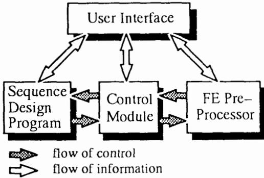
Fig. 1 The main parts of the IKBS for Forging Die Design [10].
