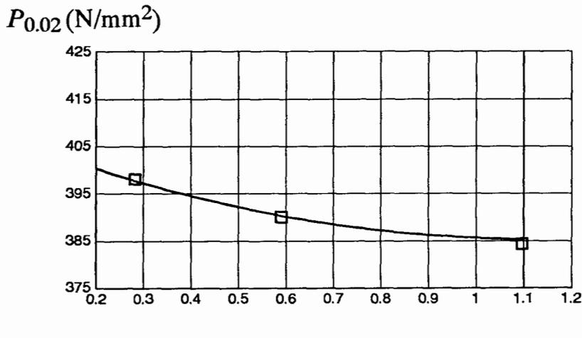
Fig. 5.7 Variation of average pressure at 2% unfilled die cavity ( $P_{0.02}$ ) with cheese ratio (height/diameter of the product  $r_c$ ) for closed–die upsetting– test No. 3
