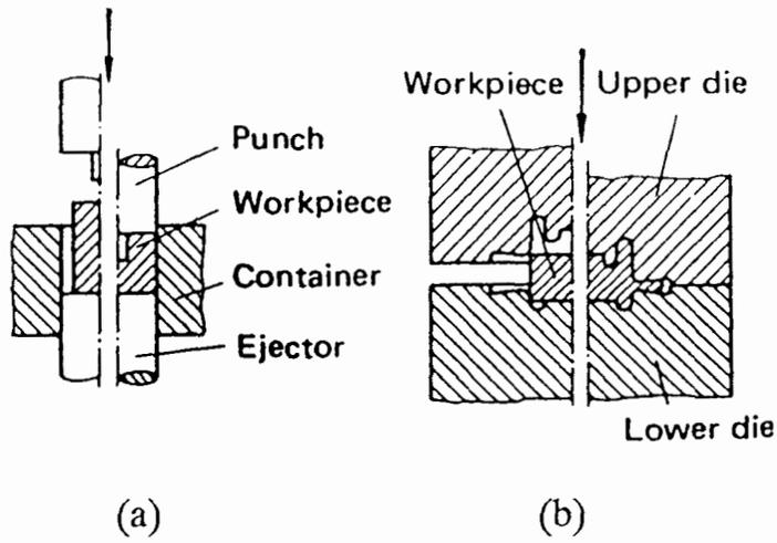
Fig. 2.1 Types of closed-die forging [6].
