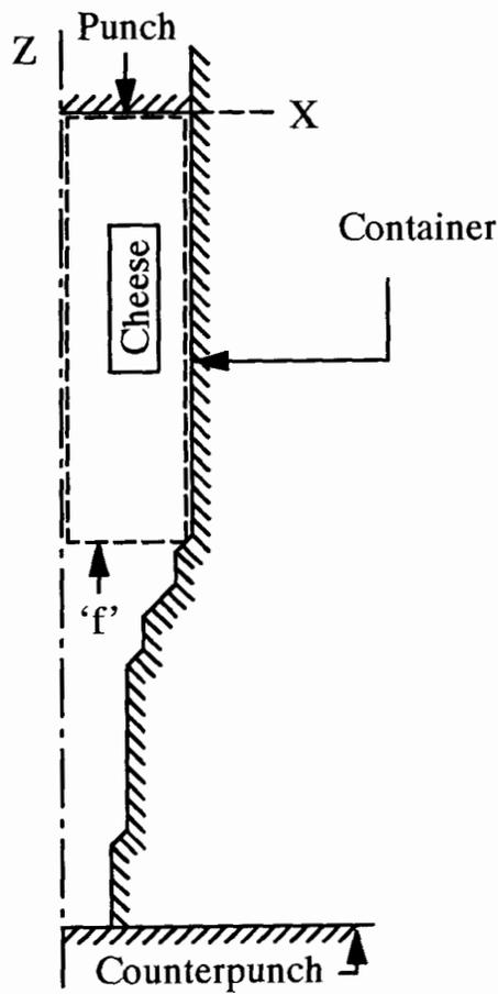
Fig. 4.14 Schematic illustration of producing 'preform' from 'cheese'
