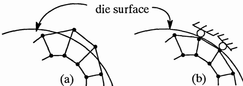
Fig. 4.4 Checking for contact between FE mesh and boundary surface
