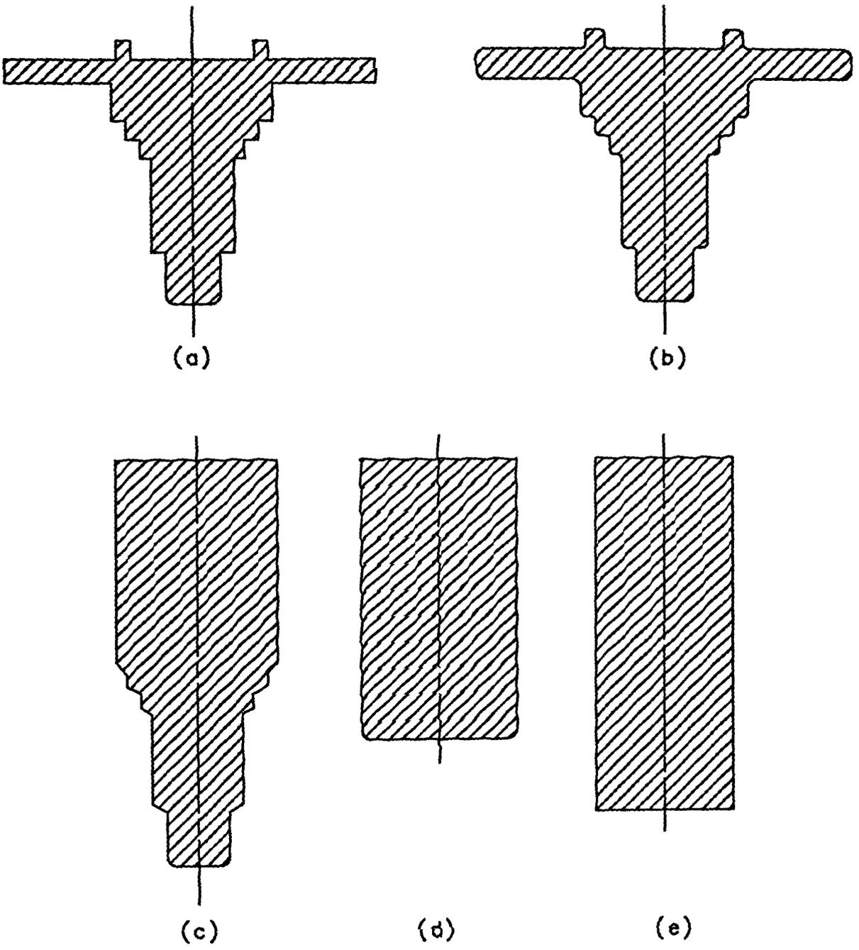
Fig. 3.5 The operational sequences for a Stub Axle [92]
