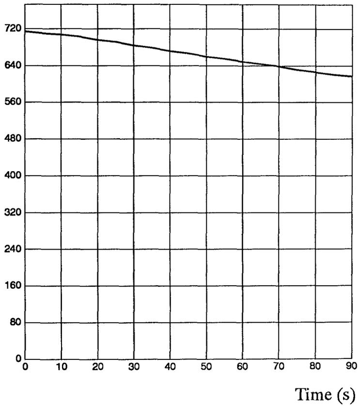
Fig. A.6 Cooling curve for near the surface of the billet
