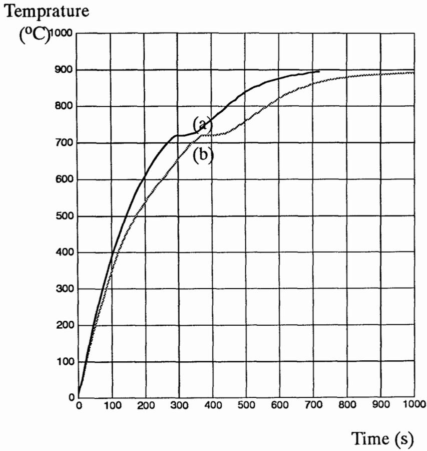
Fig. A.8 Heating curves for the centre of two examples with two different lubricants (example No. 3 in table 5.1)
