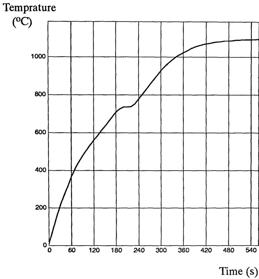
Fig. A.5 Heating curve for the centre of the billet
