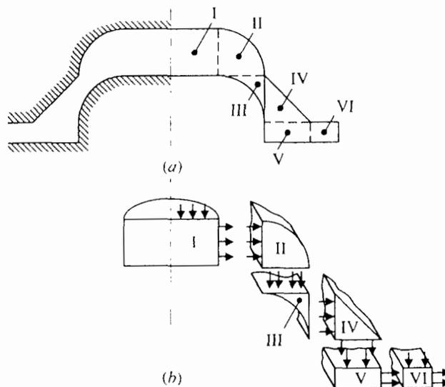
Fig 2.9 Schematic illustration of dividing half cross-section of an axisymmetric complex shape into simple shapes in UBET [40].
