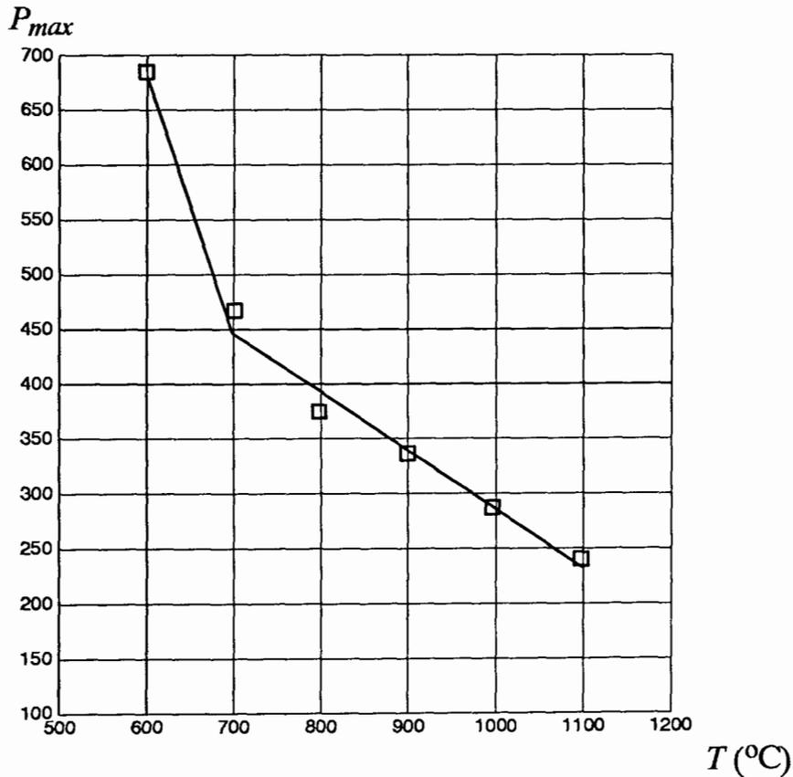
Fig. 5.14 Variation of maximum average pressure  $P_{max}$  with the workpiece pre-heat temperature  $T$  for forward extrusion- test No. 12.
