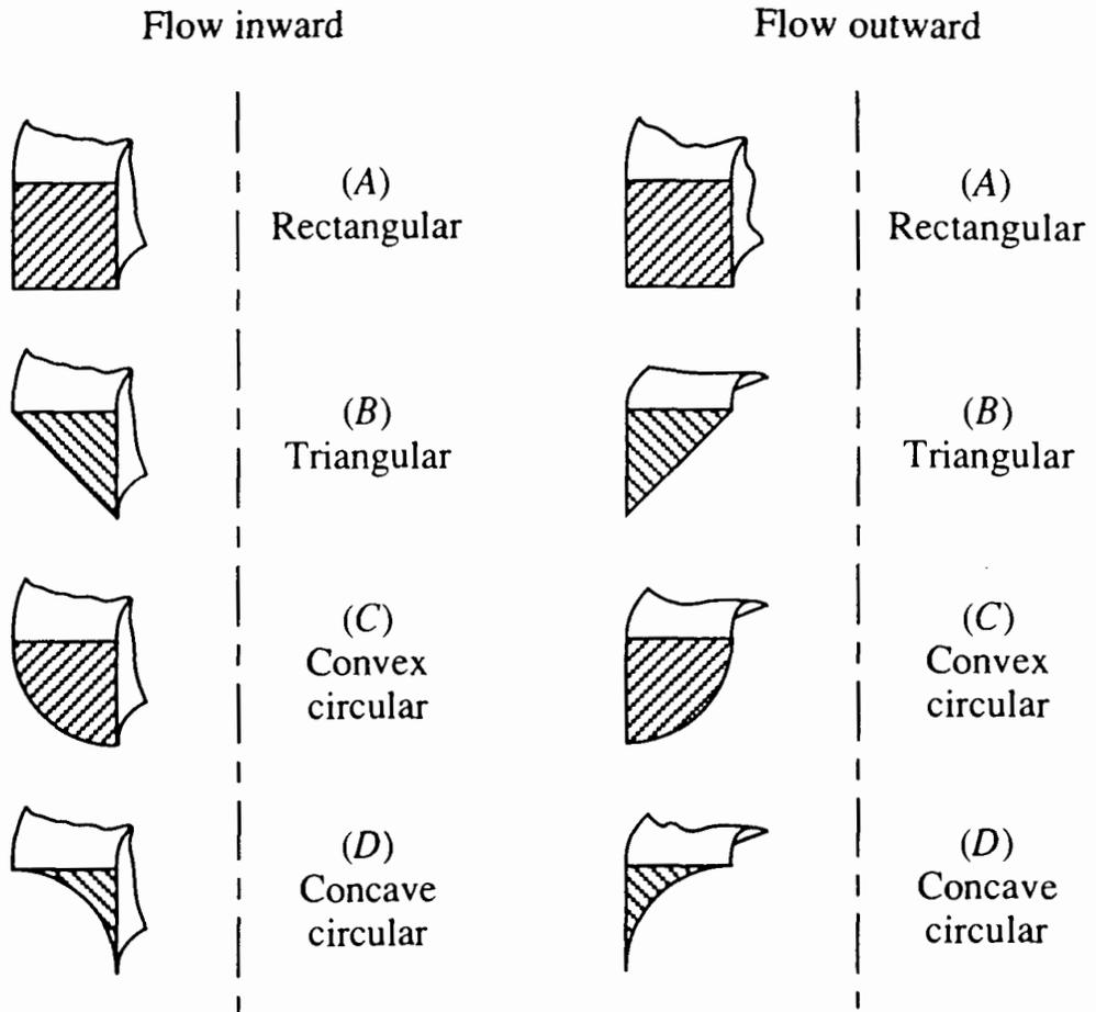
Fig. 2.8 Eight basic elemental rings in the analysis by UBET [40].
