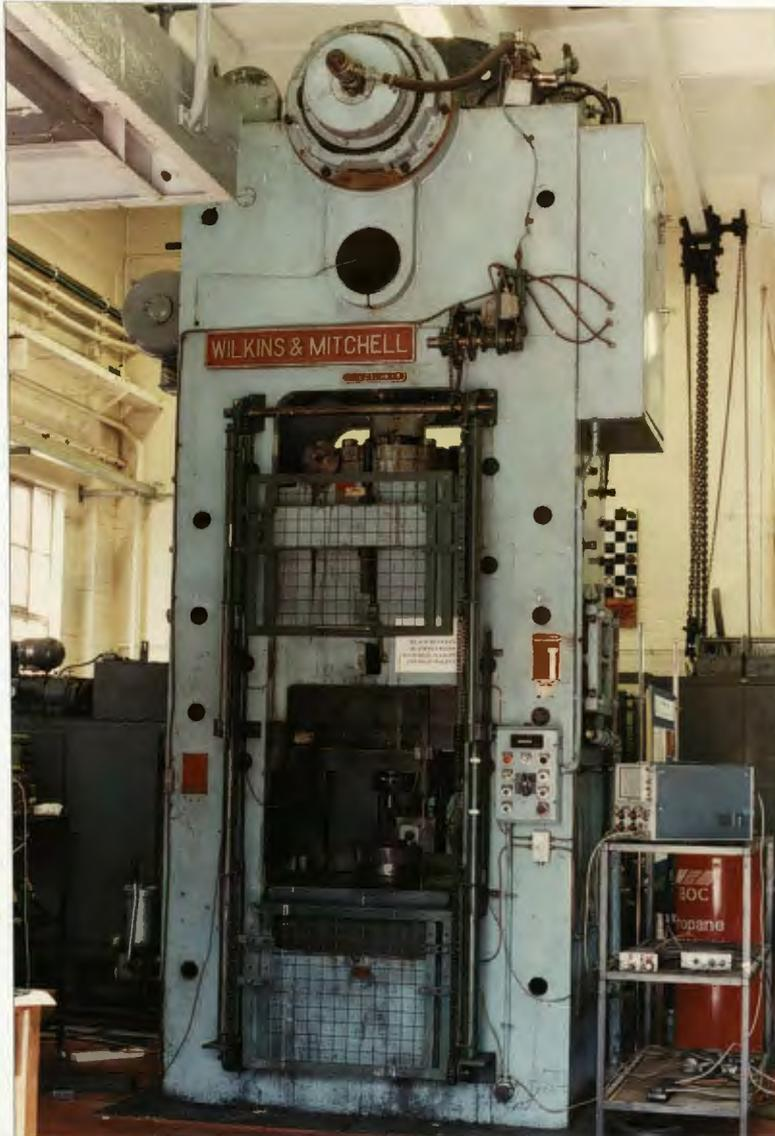
Fig. C.4 The 2000 KN mechanical press used in the experiments.
