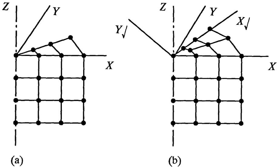
Fig. 4.9 Generating 3-D mesh for Stub Axles
