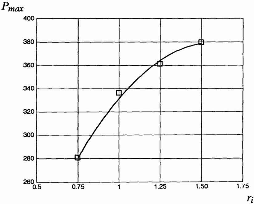
Fig. 5.13 Variation of maximum average pressure  $P_{max}$  with initial height/diameter ratio  $r_i$  for forward extrusion— test No. 9.
