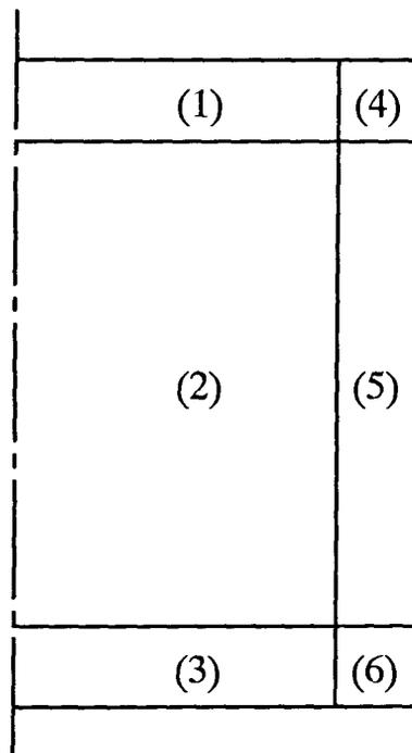
Fig. 4.10 Dividing the half cross-section of a cylindrical preform to 6 mesh areas when a fine mesh is required
