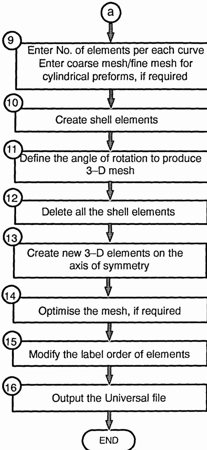
Fig. 4.8 The main actions of the mesh generation step (continued)
