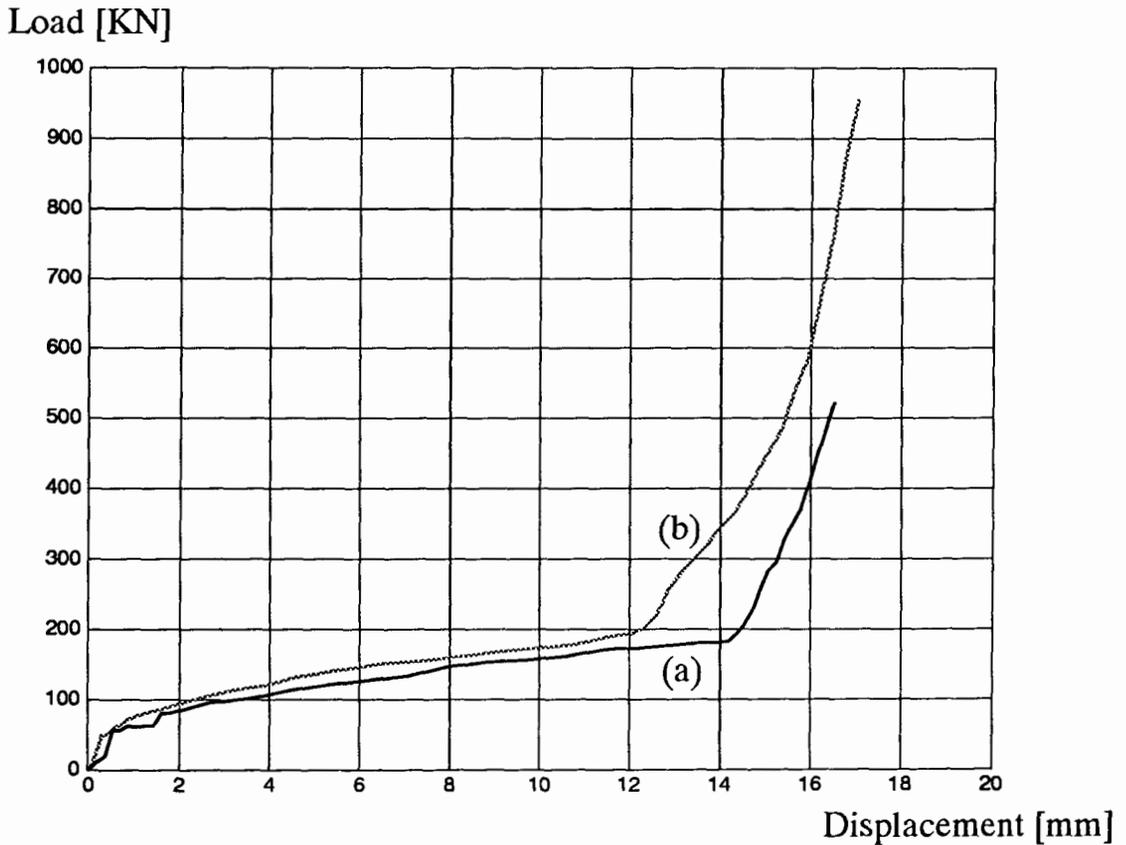
Fig. 5.11 The load-displacement curves in the two machines in closed-die upsetting.
