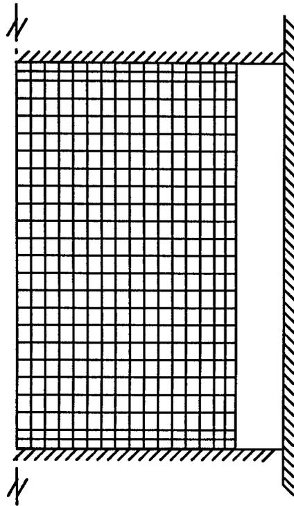
Fig. 7.1 FE mesh used to analyse the deformation (a half of the axial cross-section of billet, scale=2.5:1)
