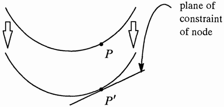
Fig. 4.5 Constraint of a node in contact with a translated die [52]
