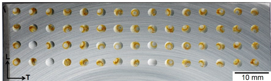
Figure 5-26 Macro photo of 304L plate surface (LT plane) deposited with arrays of \text{MgCl}_2 droplets ( \sim 2.5 mm equivalent diameter, \sim 1000 \mu\text{g}/\text{cm}^2 CDD at deposition), after 1 week exposure at 56% RH and 30 °C.
