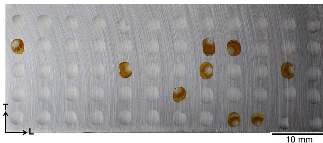
Figure 5-34 Macro photo of 316L plate surface (LT plane) with \text{MgCl}_2 droplets ( \sim 2.5 mm equivalent diameter, \sim 1000 \mu\text{g}/\text{cm}^2 CDD at deposition), following exposure at 56% RH for 1 week at 30^\circ\text{C} .
