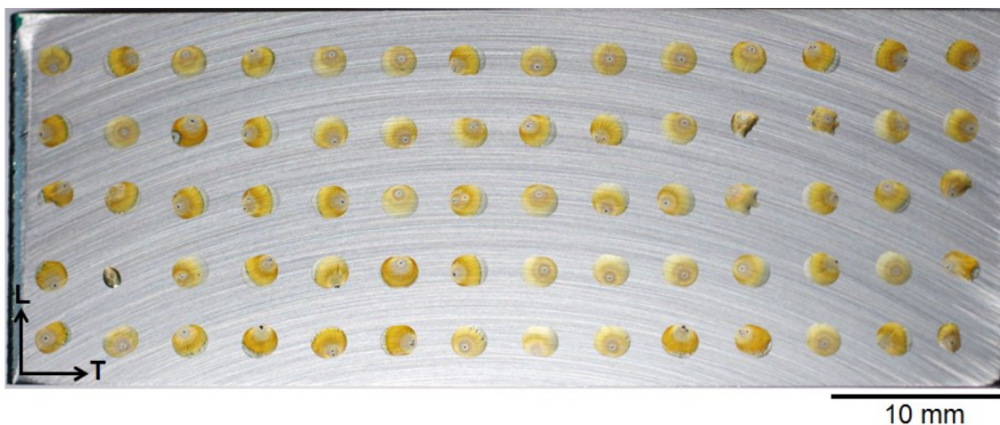
Figure 5-7 Macro photo of 304L plate surface (LT plane) with arrays of \text{MgCl}_2 droplets of \sim 2.5 mm equivalent diameter with \sim 1000 \mu\text{g}/\text{cm}^2 CDD at deposition, after 1 week exposure at 35% RH and 30^\circ\text{C} .
