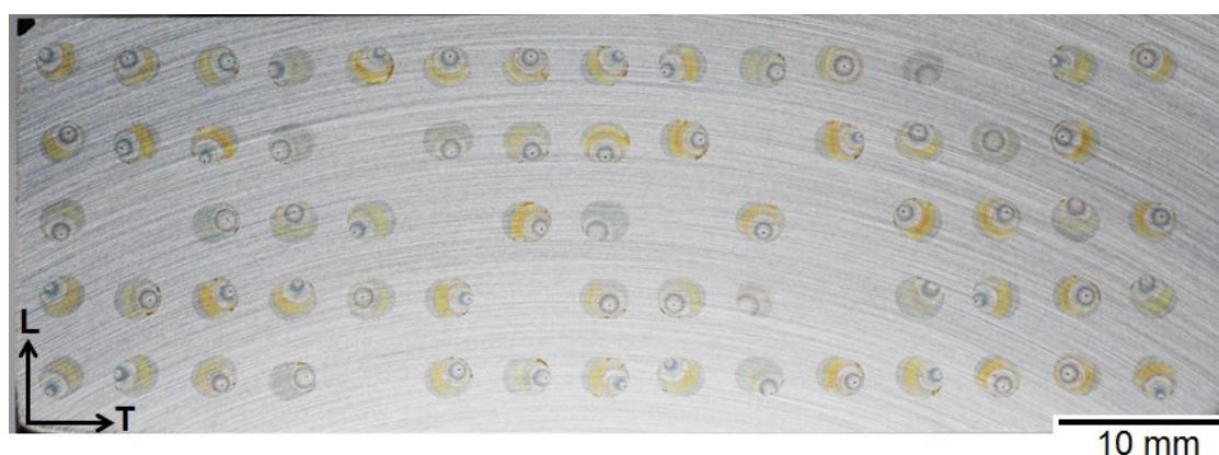
Figure 5-17 Macro photo of 304L plate surface (LT plane), after washing with DI water, with \text{MgCl}_2 droplets ( \sim 2.5 mm equivalent diameter, \sim 1000 \mu\text{g}/\text{cm}^2 CDD at deposition) after 1 day exposure at 48% RH and 30 °C.
