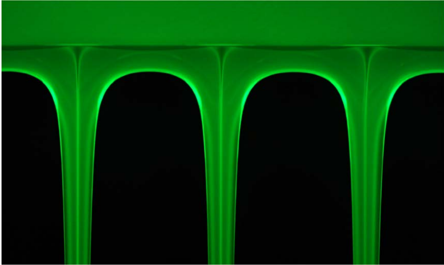
(b) Close-up of the jets, coming from the die lip. The width of the image is 3.5 cm. The flow rates are Q_1 = Q_3 = 0.55 \text{ cm}^2\text{s}^{-1} , Q_2 = 0.2 \text{ cm}^2\text{s}^{-1} .
