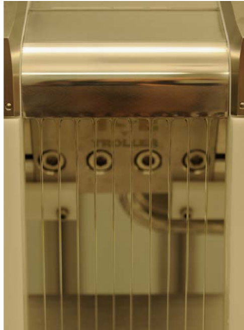
Figure 5.1: An array of liquid jets (or columns) emanating from the die lip, with a regular spacing between the centreline of each individual jet.
