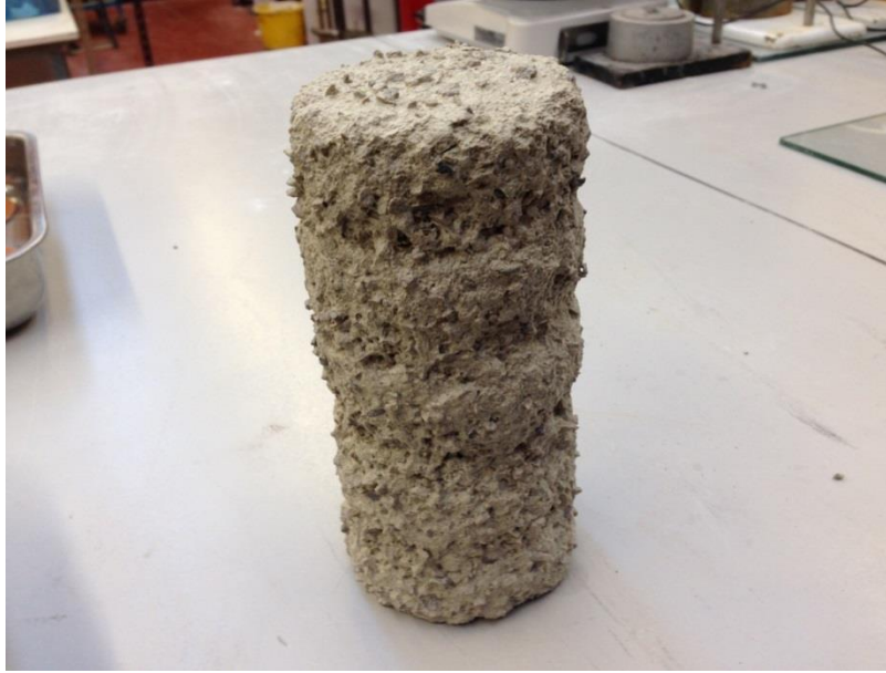
Figure 4. 26 Soil A-6 stabilised with 2%CC after 20 cycles of wetting and drying
