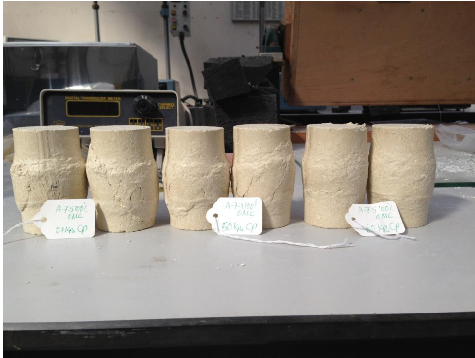
Figure 3. 18 Failure of unconsolidated untrained triaxial test for soil A-7-5 at 27, 50 and 80 kPa confining pressures at 100%OMC
