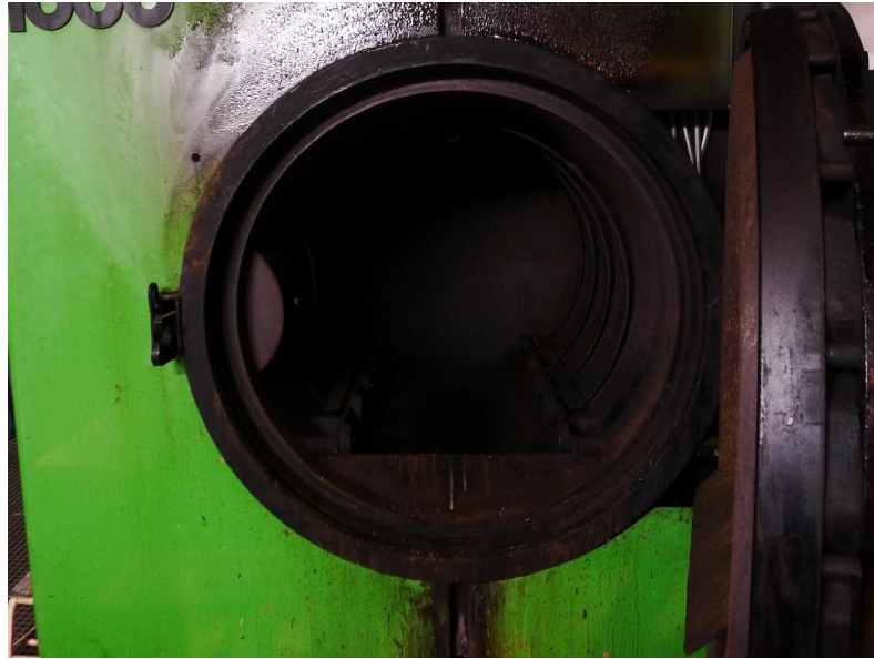
Figure 3-3: Quicklock Boilerclave™ by Leed and Bradford Boiler Company Ltd, UK. Autoclave for de-waxing in IRC laboratory. The dark and pressurised condition which is used has limit the understanding of de-waxing process.
