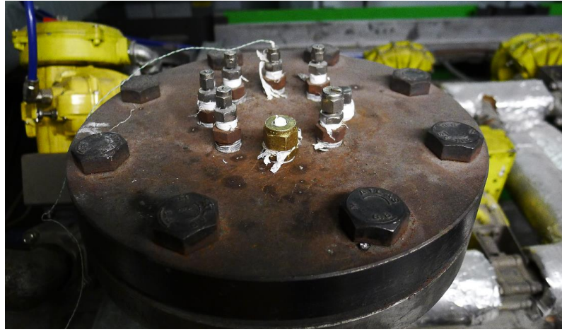
Figure 3-22: Top view of the autoclave in IRC laboratory showing the thermocouple and pressure sensor ports
