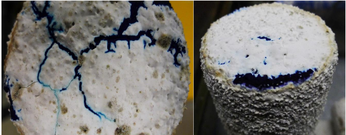
Figure 6-6: Methyl blue stain to detect cracks on the top (left) and at the edge (right) after de-waxing
