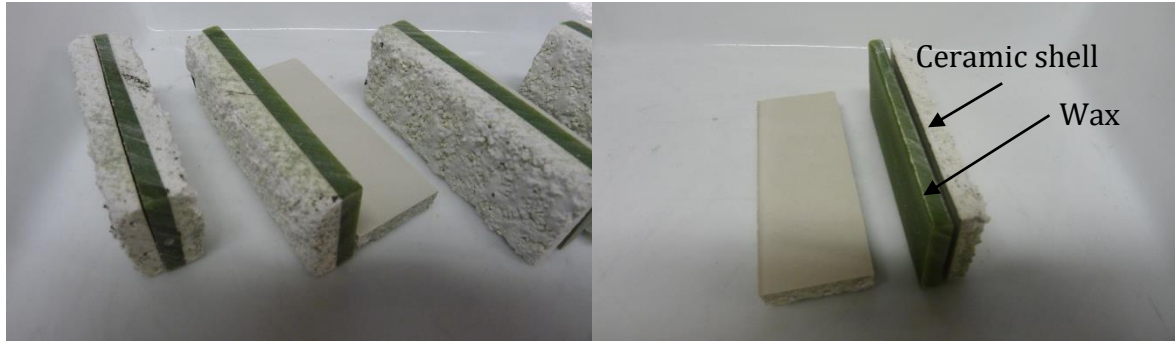
Figure 3-5: The shelled flat bar wax was cut after drying to the required test bar dimensions and then separated by cooling in a refrigerator.
