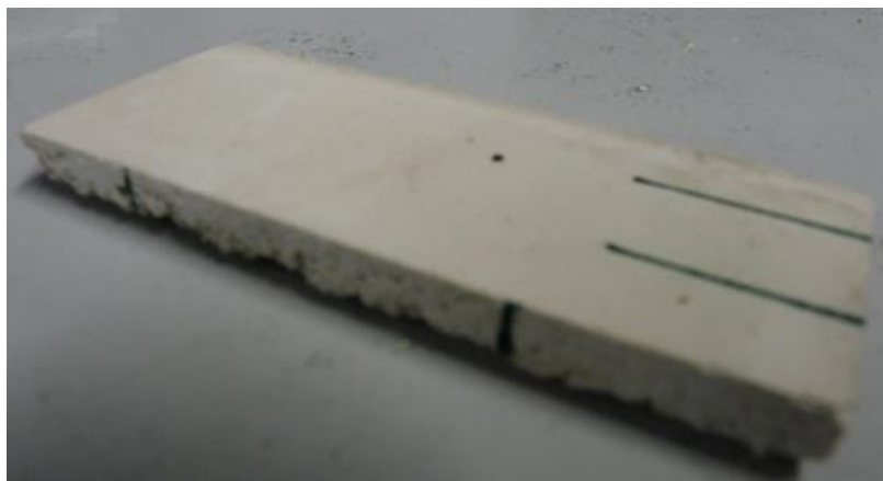
Figure 4-15: The width and thickness of each sample is noted with a line to assure the same location is being measured pre and post autoclave treatment.
