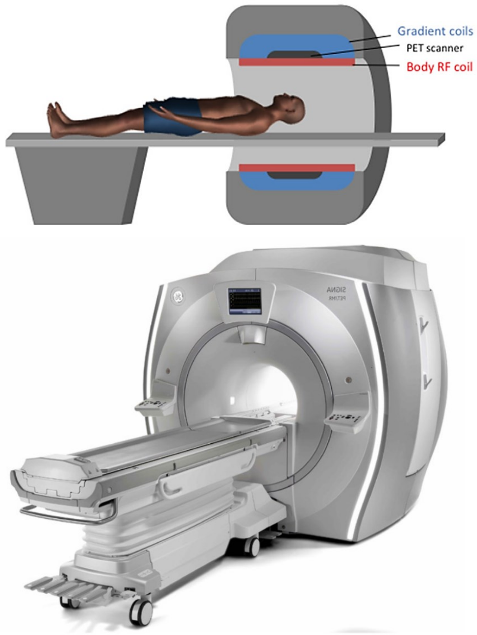
Figure 2.4. A simultaneous PET-MRI system. Upper figure is a schematic diagram of a PET-MRI system. The main magnet, Gradient coils and Radiofrequency coils (RF coils) for sending and receiving the signal are the key components of the MRI scanner, and a PET scanner is placed inside the MRI scanner. Lower figure is the GE PET-MRI system [50].
