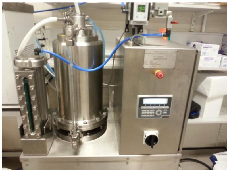
**Fig. 3.2:** A schematic diagram (a) and a photograph (b) of the pilot-scale rotating membrane emulsification system used within this thesis.
