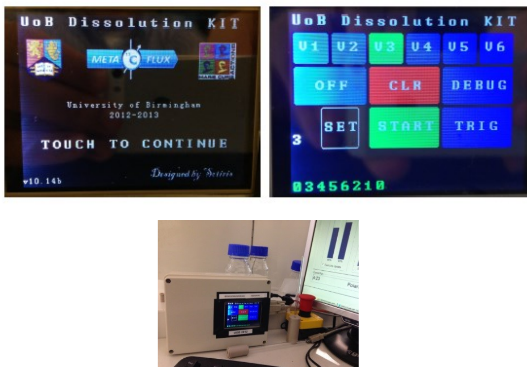
Figure 3.11 – Photograph of the Touch Interface splash and operation screen
