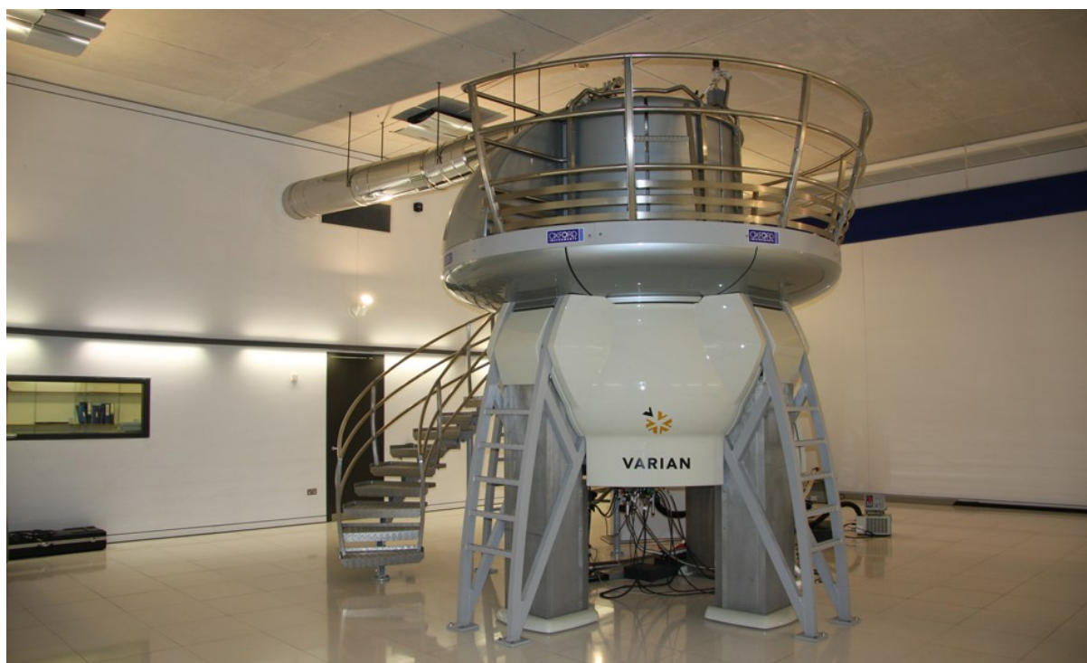
Figure 1.6 - The 900MHz magnet found in HWB-NMR in Birmingham
