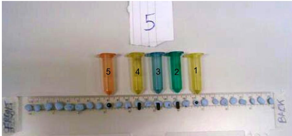
Figure 4.18. Photo of set up for resolution test 5. Similar set up to test 4 but with source 5 placed 30 mm away from the rest of the sources which are separated by 20 mm.
