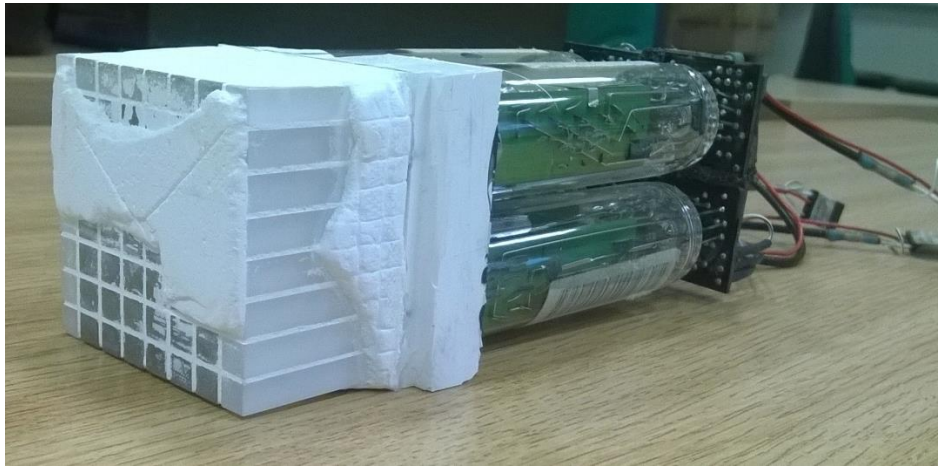
Figure 2.18. Photo of a detector block coupled with four PMTs.
