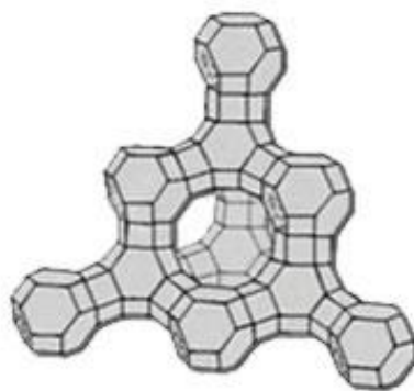
Figure 2.39. Figure showing 1 the tetrahedral structure of silica and alumina that make up Zeolite 13X. This structure contains consistent pore diameters of 0.1 nm.
