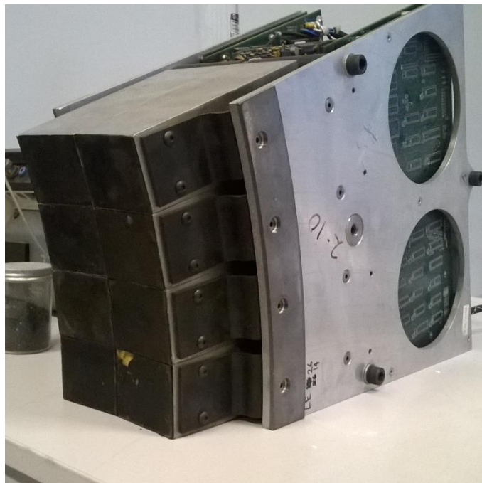
Figure 2.19. Photo of a bucket which consists of 2 x 4 blocks of detectors.
