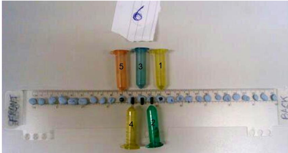
Figure 4.21. Photo of set up for resolution test 6. All five sources are spaced 10 mm apart.
