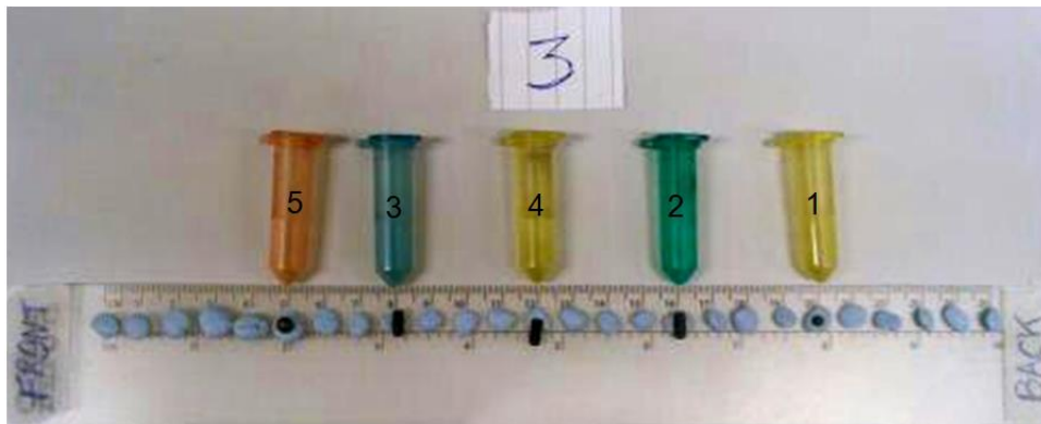
Figure 4.12. Photo of set up for resolution test 3. The blue marker indicates the location of source 3 and the green marker indicates the location of source 2.
