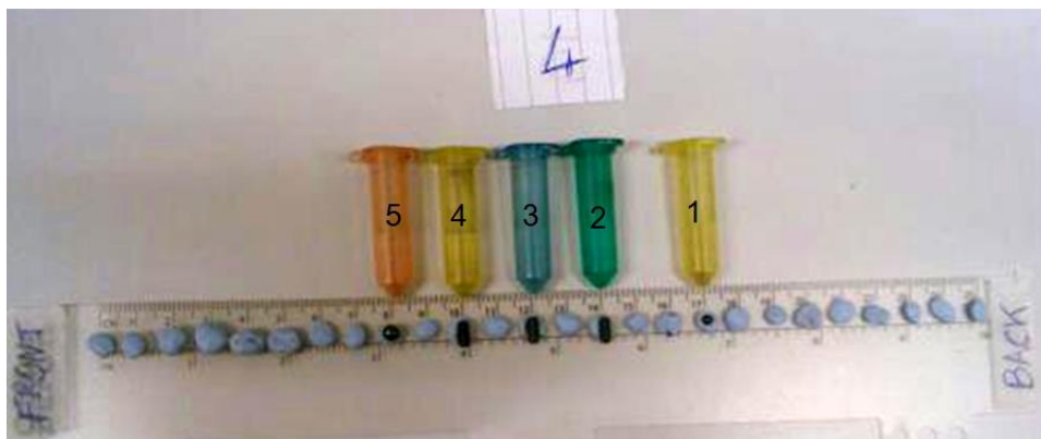
Figure 4.15. Photo of the set up for resolution test 4. The sources have been re-ordered to 5, 4, 2, 3 and 1 and moved closer to each other, separated by 20 mm with source 1 positioned 30 mm away.
