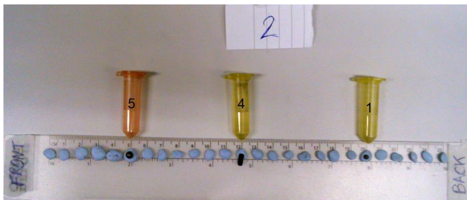
Figure 4.9. Photo of set up for resolution test 2. The central yellow marker indicates the position of source 4. Source 4 is a spherical source and source 5, also identified by a yellow marker, is a pellet.
