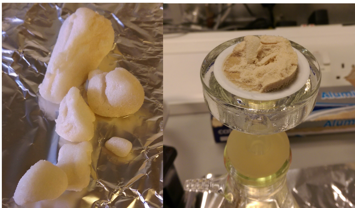
Figure 4.5: Abraded XPS foam after contact and foam particles filtered out of leachate after a contact period of 48 h in single batch experiments.
