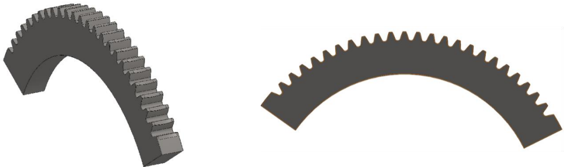
Figure 4-28. 3D design of the worm wheel part.
