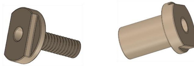
Figure 4-38. 3D design of the assembly of the screw 1 (left) and nut 2 (right).
