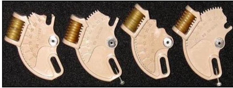
Figure 3-4. Mechanical failure at distal arcuate hinge (adapted from (Lahiri et al. , 2007)).
