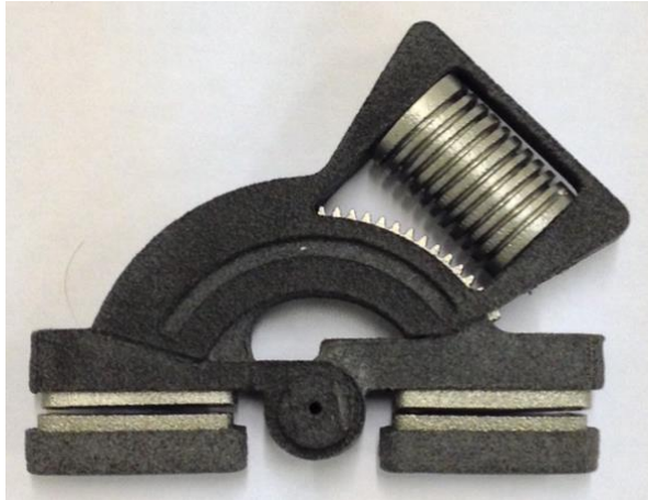
Figure 5-11. External dynamic protractor hinge fixator working model.
