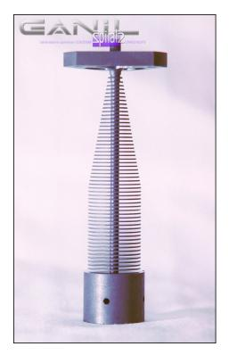
Figure 3.3: Photograph of the SPIRAL carbon target for the production of radioactive nuclei. [52]
