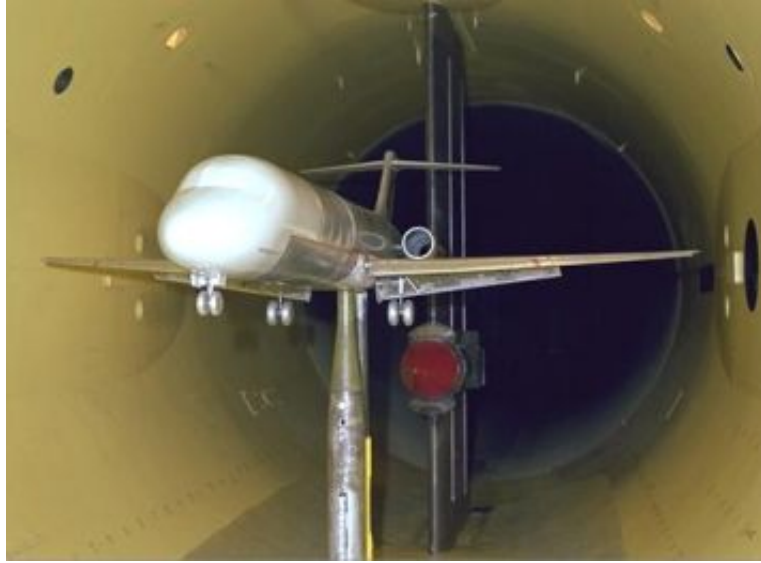
Figure 2.1: Photo of a wind-tunnel experiment involving a scale model of an aeroplane (source: "Windkanal" by JeLuF - http://en.wikipedia.org/wiki/Image:Windkanal.jpg . Licensed under Creative Commons Attribution-Share Alike 3.0 via Wikimedia Commons).
