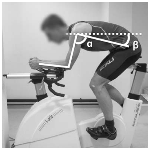
Figure 5.1 Definition of torso angle \beta and shoulder angle \alpha . The torso angles analysed were 0,8,16 and 24° relative to the ground, whilst the shoulder angle remained constant. The head position can affect the aerodynamic drag (Lukes et al., 2005). However, for obvious safety reasons cyclists have to maintain their head upright and therefore the current model assumes this position is adopted.
