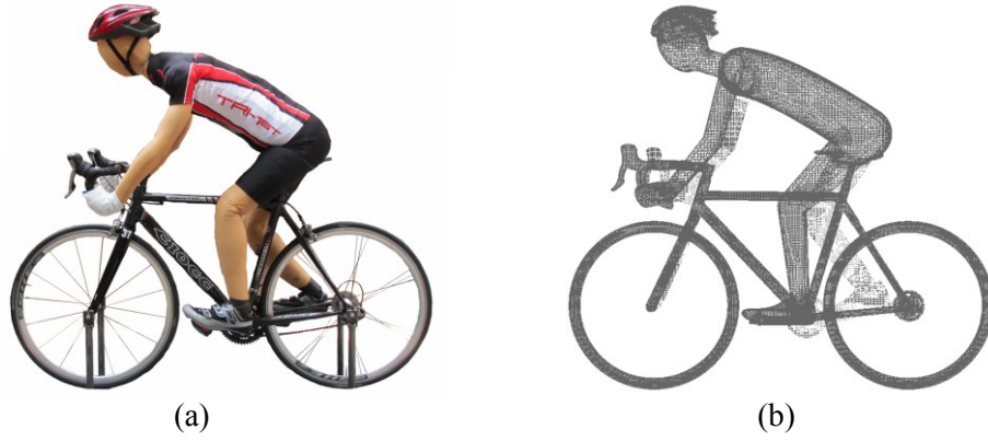
Figure 7.2 (a) Full-scale bicycle and mannequin used in wind tunnel experiments and (b) geometry of the bicycle and cyclist in simulations.
