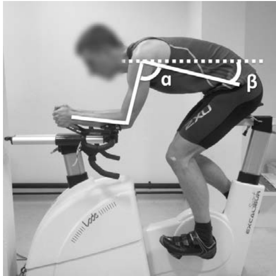
Figure 2.1 Definition of the torso angle, \beta , and upper arm angle, \alpha
